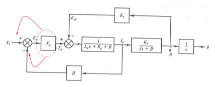
$$G_1(s) = \frac{1/(L_a s + R_a + R)}{1 + K_a R/(L_a s + R_a + R)} = \frac{1}{L_a s + R_a + R + K_a R}$$
