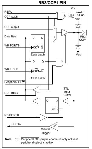
FIGURE 5-11: BLOCK DIAGRAM OF
