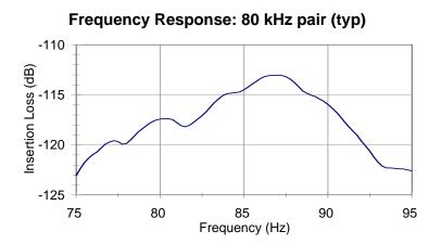
The plot at left shows an estimate of the frequency response curve for two identical units, one driven as transmitter, the other acting as a receiver. The spectrum of the received signal was divided by that of the drive signal and gain stage, giving the overall insertion loss as a function of frequency (measured at 30 cm distance, in air).
