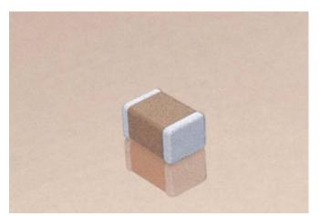
X7R formulations are called "temperature stable" ceramics and fall into EIA Class II materials. X7R is the most popular of these intermediate dielectric constant materials. Its temperature variation of capacitance is within  $\pm 15\%$  from -55°C to +125°C. This capacitance change is non-linear.
