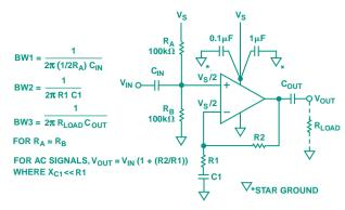
Figure 1. A potentially unstable single-supply op amp circuit.
