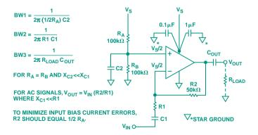
Figure 3. A decoupled single-supply inverting amplifier circuit.
