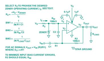
Figure 5. An inverting single-supply amplifier using Zener-diode biasing.
