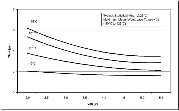
FIGURE 18-36: TYPICAL HFINTOSC START-UP TIMES vs. VDD OVER TEMPERATURE
