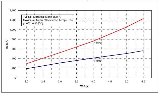
FIGURE 18-7: IDD vs. VDD (LP MODE)
