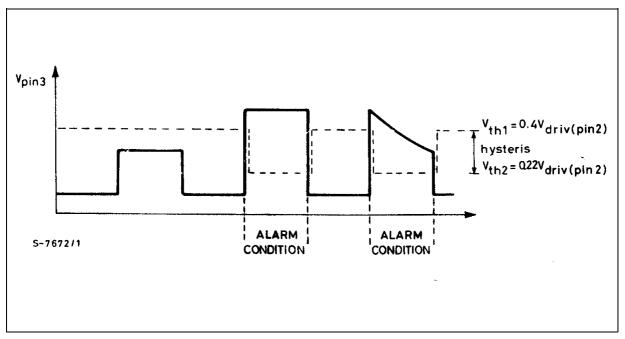
Figure 1b: Pin 8 High; Alarm with Input Voltage < Threshold.
