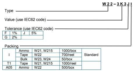
For CECC released product state on order the CECC number and style. Example: **W22-3K3JI CECC40201-002 JB** For SnPb finish instead of Pb-free replace the packing suffix with **PB**. Example: **W22-3K3JPB**
