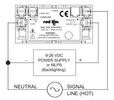
Optional backlight versions of the CUB4 require an external 9-28 VDC power supply. The external supply is connected between the V+ and Common terminals as shown in the drawing.
