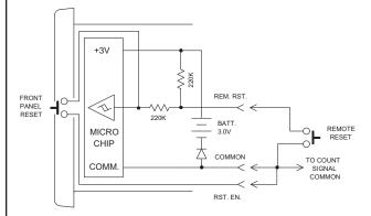
Connecting a wire from the "RST. EN." (Reset Enable) Input terminal to Common will enable the front panel Reset button. When Remote Reset is required, a wire is connected from the "REM. RST." input terminal to Common. Pulling this input low causes the counter to reset. The "REM. RST." can be pulled low by either a mechanical switch or solid-state transistor switch. Switch load and leakage are the same as for "L.S. CNT." Input above.
