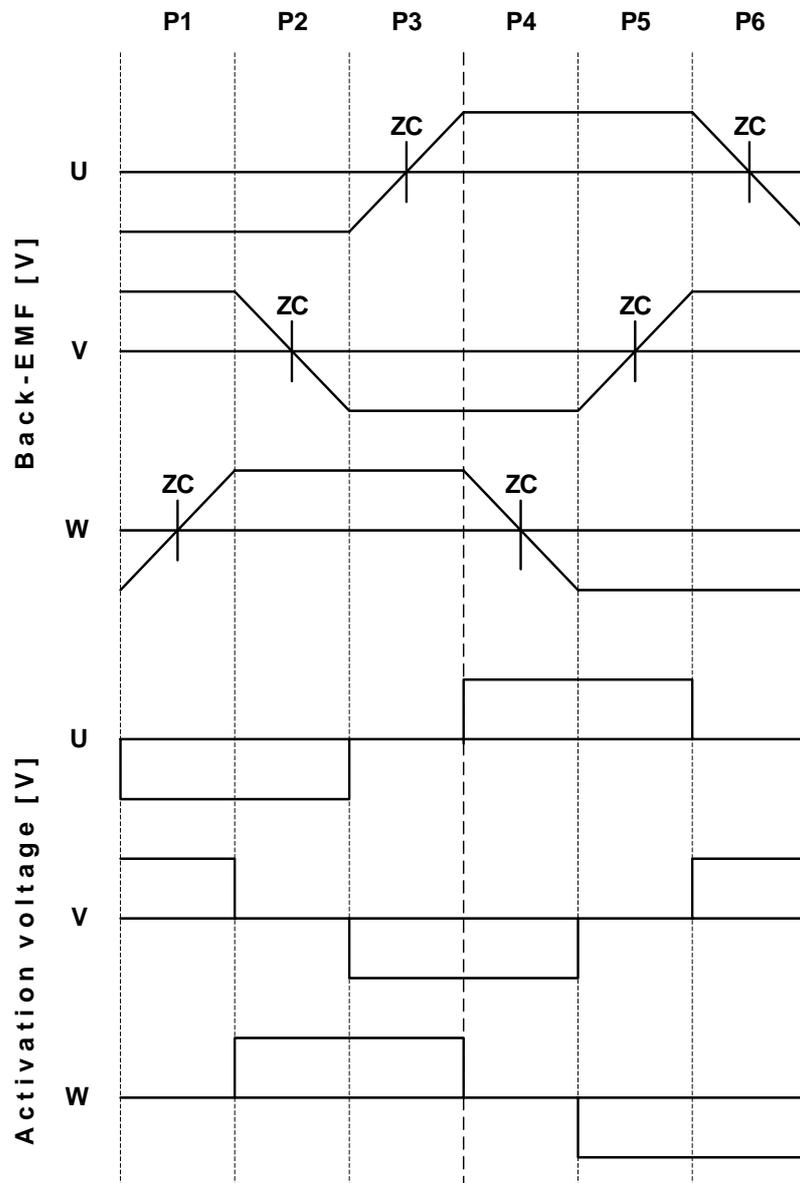
The floating phase, where the zero crossing must be detected, changes for every commutation step. One ADC channel for each phase winding is needed to detect zero crossings.
