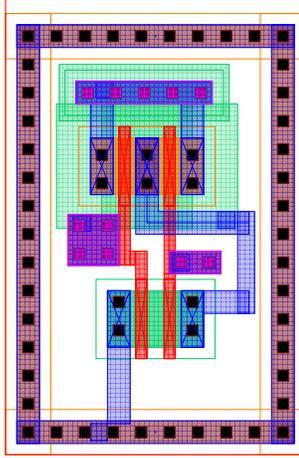
Figure 52: CMOS 2 Input nand
