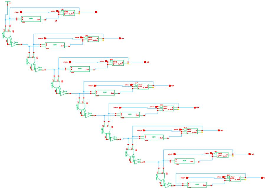
Figure 16: 8-bit synchronous counter
