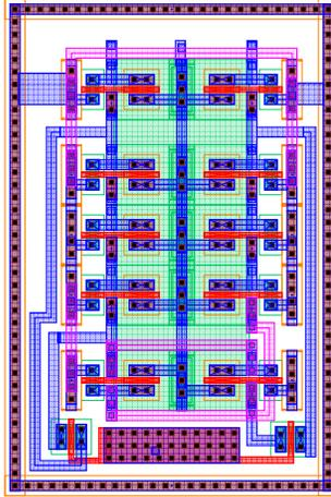
Figure 40: 1GHz Frequency Divide By 2
