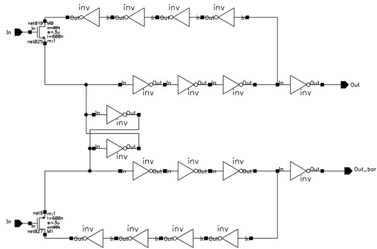
Figure 20: 400 MHz Frequency Divider
