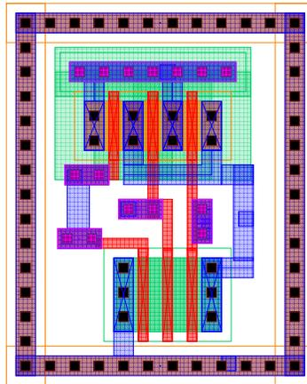
Figure 53: CMOS 3 Input nand
