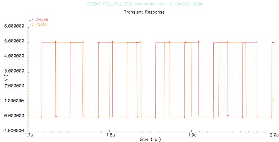
Figure 30: Output of PFD DPLL with Frequency Divider Divided by 2
