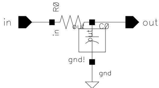
Figure 21: RC Low Pass Filter
