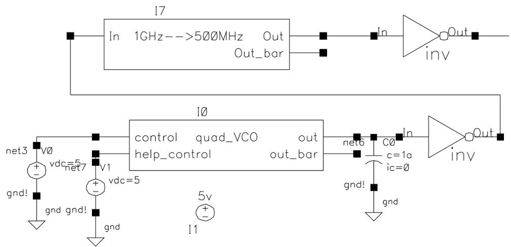
Figure 24: 1GHz Test Oscillator Schematic
