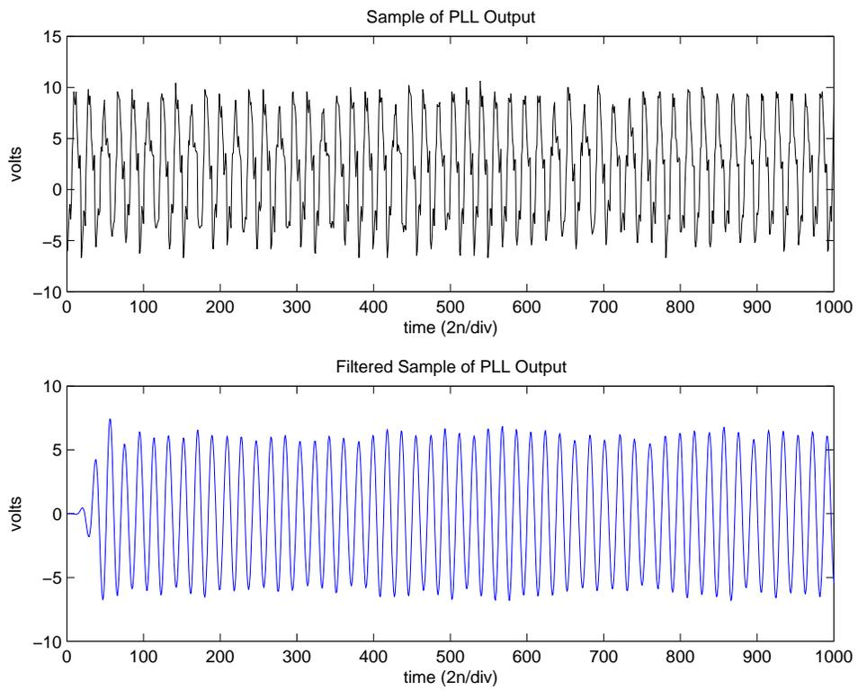
Figure 38: Output Waveform from 30MHz DPLL
