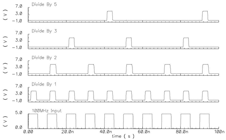
Figure 32: Programmable Counter Divide Simulation
