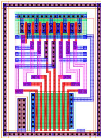
Figure 54: CMOS 8 Input nand
