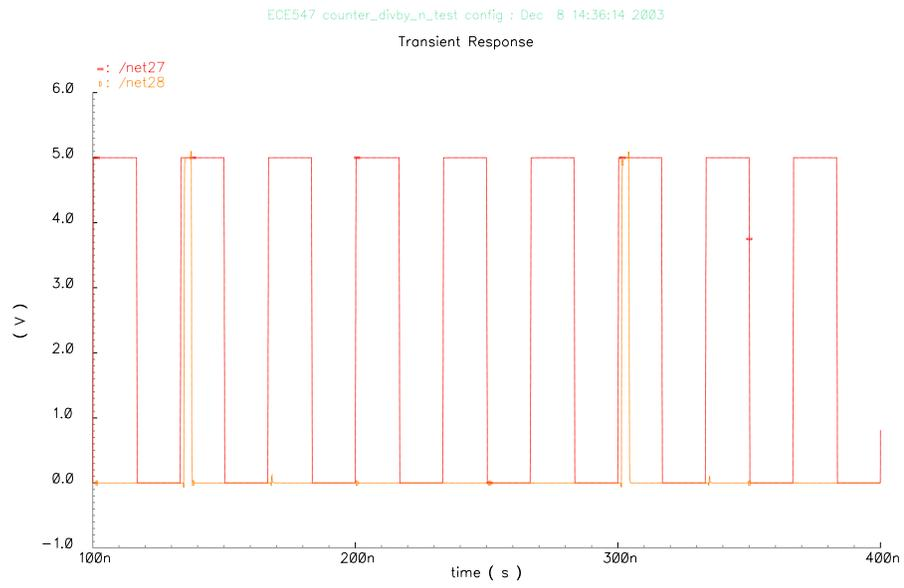
Figure 29: Output of Frequency Divider Divided by 5
