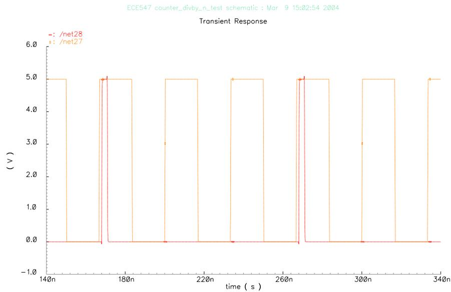
Figure 28: Output of Frequency Divider Divided by 3
