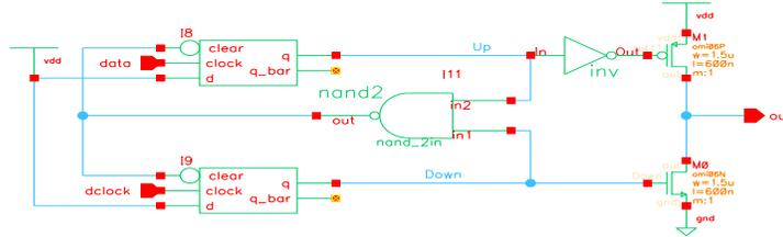
Figure 11: Phase Frequency Detector
