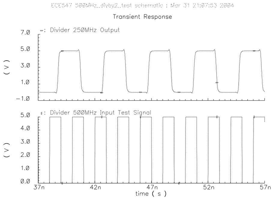
Figure 35: 500MHz Frequency Divider
