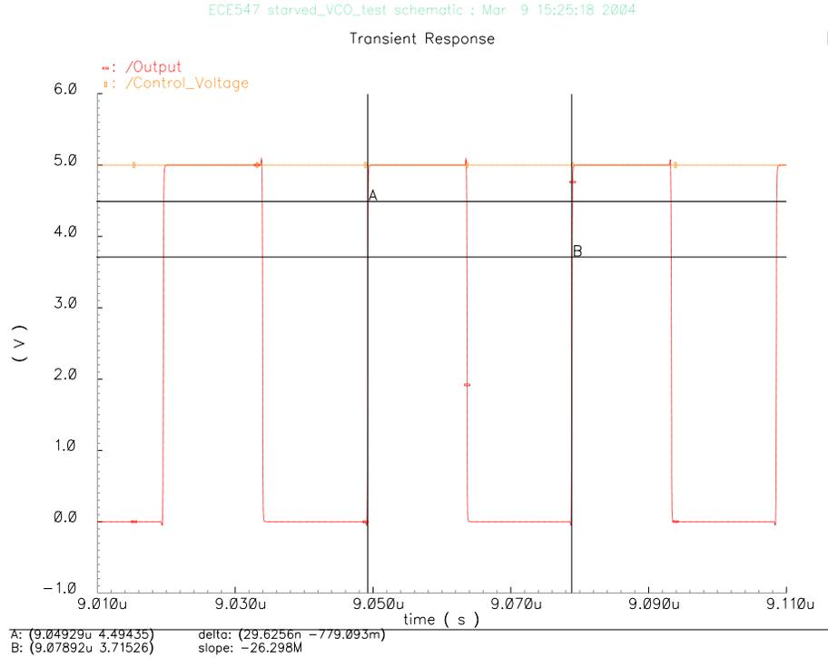
Figure 26: Output of VCO at Control Voltage of 5V
