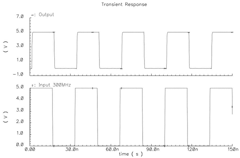
Figure 33: 300MHz Buffer Driving 40pF Load
