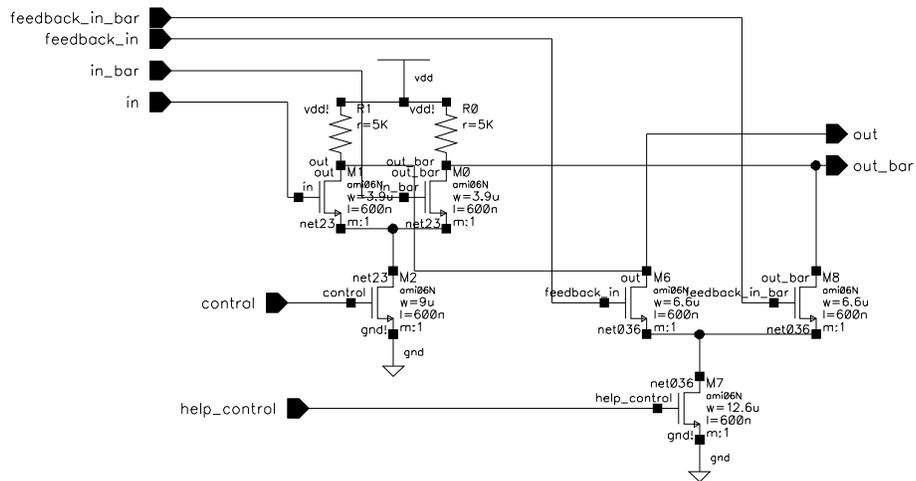
Figure 19: Quadrature Output VCO Cell
