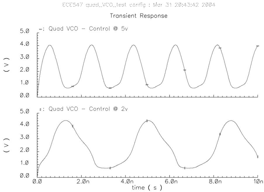
Figure 34: Quad VCO Oscillations at Control Voltage Extremes
