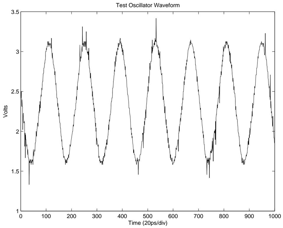
Figure 37: Test VCO Output when Control is 3v
