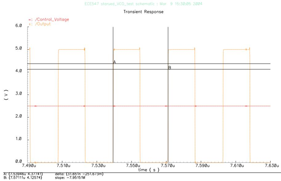
Figure 27: Output of VCO at Control Voltage of 2.5V
