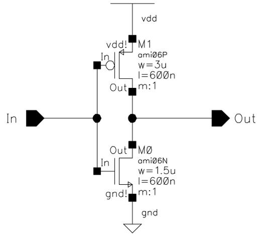
Figure 2: Minimum sized CMOS inverter
