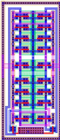
Figure 41: 500MHz Frequency Divide By 2
