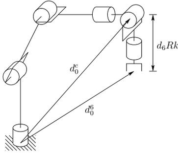
Figure 4.1: Kinematic decoupling.
