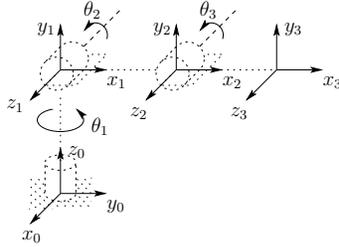
Figure 3.1: Coordinate frames attached to elbow manipulator.
