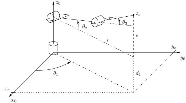
Figure 4.2: Elbow manipulator.
