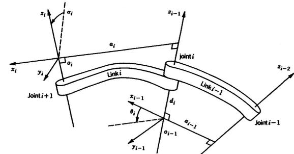
Figure 3.4: Denavit-Hartenberg frame assignment.
