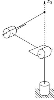
Figure 4.4: Singular configuration.
