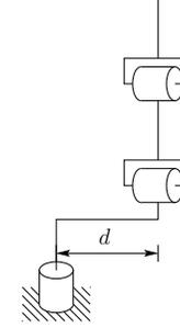
Figure 4.5: Elbow manipulator with shoulder offset.
