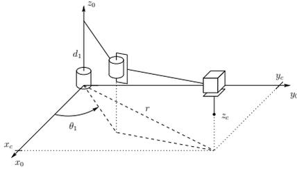
Figure 4.11: SCARA manipulator.
