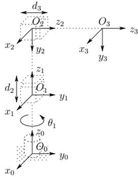
Figure 3.7: Three-link cylindrical manipulator.
