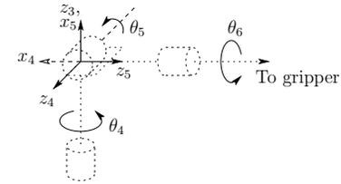
Figure 3.8: The spherical wrist frame assignment.
