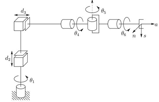
Figure 3.9: Cylindrical robot with spherical wrist.
