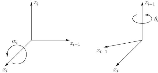
Figure 3.3: Positive sense for  $\alpha_i$  and  $\theta_i$ .
