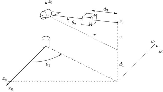
Figure 4.10: Spherical manipulator.
