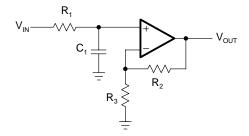
Figure 16-12. First-Order Noninverting Low-Pass Filter
