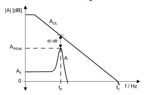
Figure 16–53. Open-Loop Gain (A<sub>OL</sub>) and Filter Response (A)
