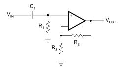
Figure 16–25. First-Order Noninverting High-Pass Filter
