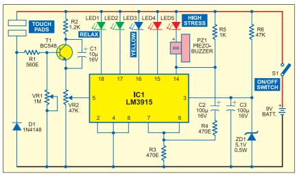
Fig. 1: Circuit of the stress meter
