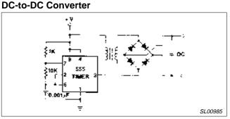
Figure 32. DC-to-DC Converter
