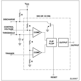
Figure 4. Monostable Operation
