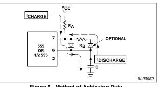
Figure 6. Method of Achieving Duty Cycles Less Than 50%
