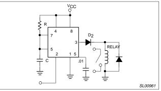
Figure 8. Driving High Q Inductive Loads
