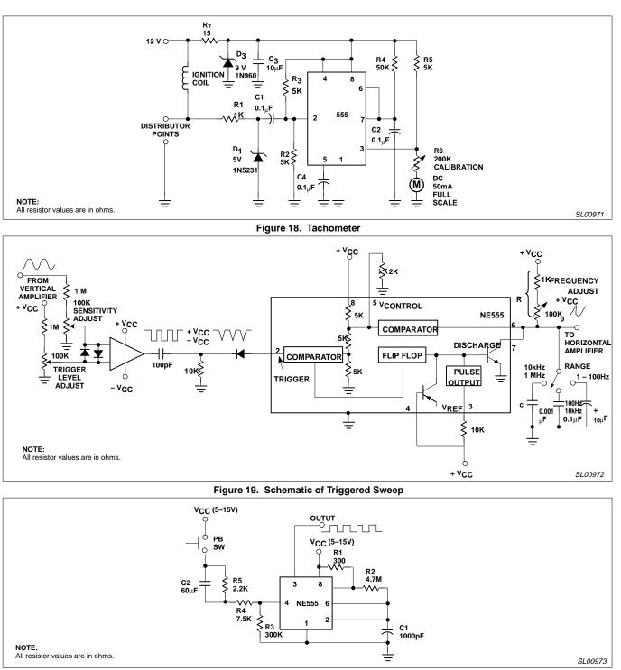
Figure 20. Square Wave Tone Burst Generator
