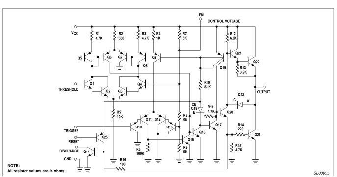
Figure 2. Schematic of 555 or 1/2 556 Dual Timer
