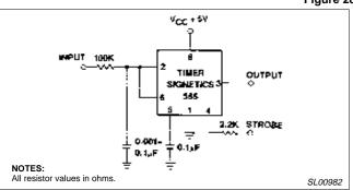
Figure 29. Low Cost Line Receiver
