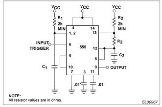
Figure 14. Tone Burst Generator the time between pulses to around twenty minutes.
