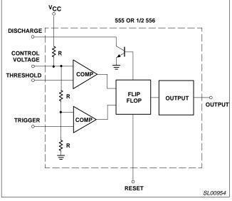
Figure 1. 555/556 Timer Functional Block Diagram
