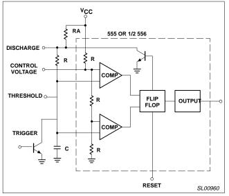
Figure 7. Time Delay Operation
