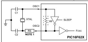
Note 1: A series resistor may be required for some crystals.
