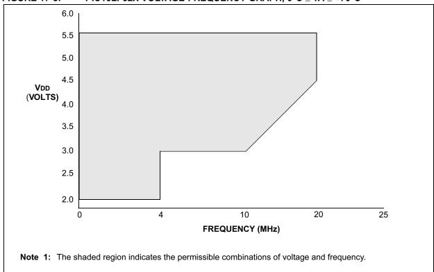
FIGURE 17-4: PIC16LF62X VOLTAGE-FREQUENCY GRAPH,  $-40^{\circ}\text{C} \leq \text{TA} < 0^{\circ}\text{C}, +70^{\circ}\text{C} < \text{TA} \leq 85^{\circ}\text{C}$
