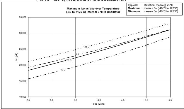
FIGURE 18-25: TYPICAL IDD VS VDD OVER TEMPERATURE (-40 TO +125°C) INTERNAL 37 kHz OSCILLATOR
