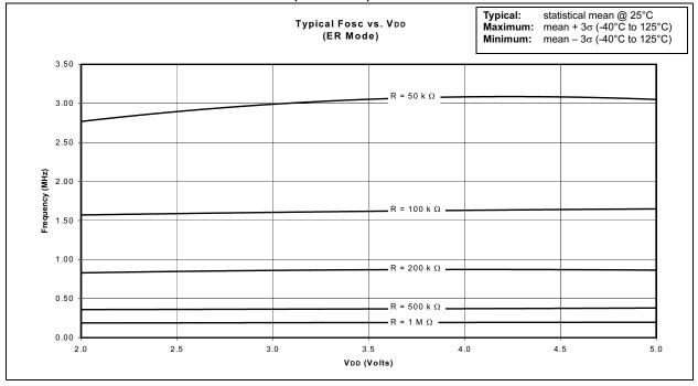
FIGURE 18-8: TYPICAL INTERNAL RC FOSC VS VDD TEMPERATURE (-40 TO 125°C) INTERNAL 4 MHz OSCILLATOR
