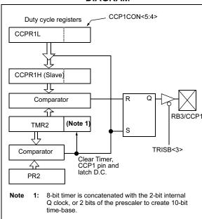
A PWM output (Figure 11-3) has a time-base (period) and a time that the output stays high (duty cycle). The frequency of the PWM is the inverse of the period (1/period).
