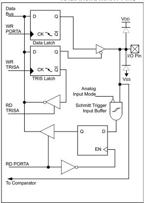
FIGURE 5-2: BLOCK DIAGRAM OF RA2/VREF PIN
