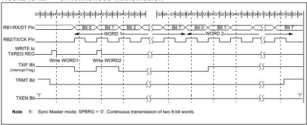
FIGURE 12-13: SYNCHRONOUS TRANSMISSION (THROUGH TXEN)
