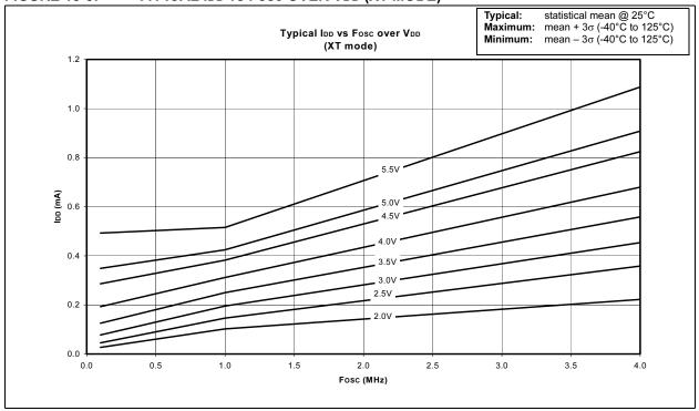
FIGURE 18-4: TYPICAL IDD VS FOSC OVER VDD (XT MODE)
