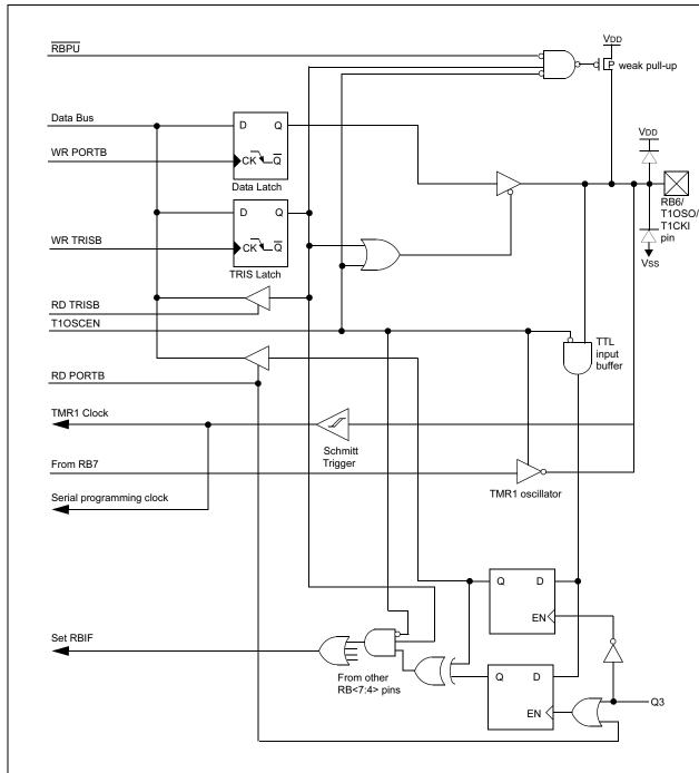
FIGURE 5-14: BLOCK DIAGRAM OF RB6/T1OSO/T1CKI PIN
