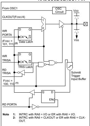
FIGURE 5-7: BLOCK DIAGRAM OF RA7/OSC1/CLKIN PIN
