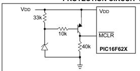
Note 1: This circuit will activate RESET when VDD goes below (Vz + 0.7V) where Vz = Zener voltage.
