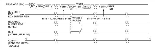
Note 1: This timing diagram shows an address byte followed by an data byte. The data byte is not read into the RCREG (receive buffer) because ADEN was not updated (still = 1) and Bit 8 = 0.
