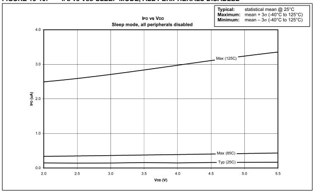
FIGURE 18-11: Albod vs Voh OVER TEMPERATURE (-40 to 125°C)
