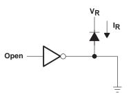
Figure 6. I<sub>R</sub> Test Circuit
