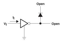
Figure 3. I<sub>I(on)</sub> Test Circuit
