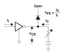
Figure 5. h<sub>FE</sub>, V<sub>CE(sat)</sub> Test Circuit
