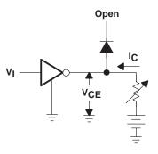
Figure 4. VI(on) Test Circuit
