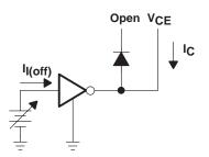
Figure 2. Il(off) Test Circuit
