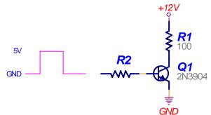
Note: The transistor isn't a perfect switch. When off there is a small current that flows (~50nA for the 2N3904) and when on it has a small voltage drop (~0.2V depending on the collector & base currents).
