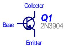
The schematic representation of a transistor is shown to the left. Note the arrow pointing down towards the emitter. This signifies it's an NPN transistor (current flows in the direction of the arrow). See the datasheet at: <u>www.fairchildsemi.com</u>.
