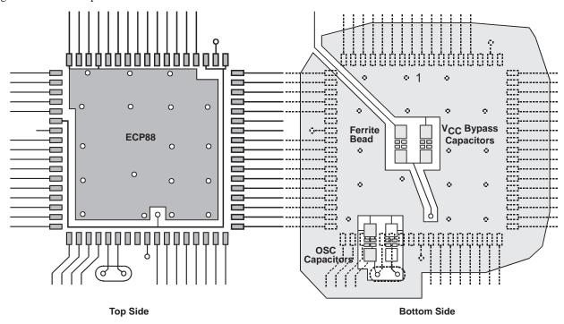
Figure 4. Microcomputer Ground
