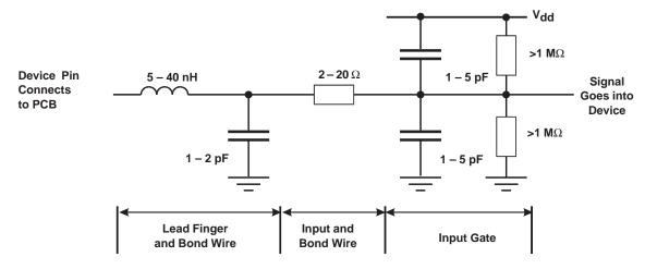
Figure 11. MOS Buffer Simplified Schematic
