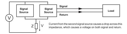
Common-mode noise is the noise voltage that travels down both the signal and return caused by a voltage drop across a shared impedance. Ground bounce on outputs is an example of common-mode noise.
