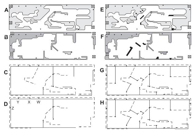
Figure 8. Gridding of Ground Fills and Traces to Form a Ground Plane
