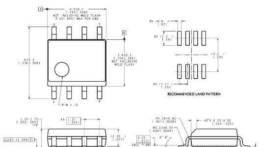
CONTROLLING DIMENSION IS MILLIMETER
