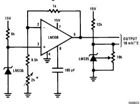
\*Adjust for 2.7315V at output of LM308
