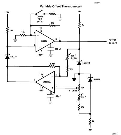
†Adjust for zero with sensor at 0°C and 10T pot set at 0°C
