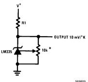
\*Calibrate for 2.982V at 25°C
