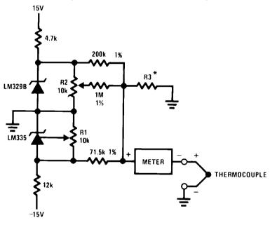
\*Select R3 for proper thermocouple type
