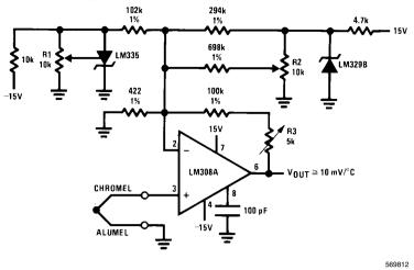
Terminate thermocouple reference junction in close proximity to LM335.
