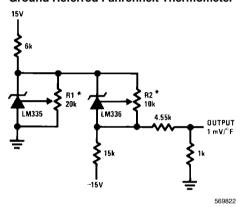
\*Adjust R2 for 2.554V across LM336. Adjust R1 for correct output.
