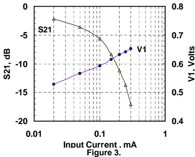
If the diodes are driven from a voltage source (not shown), the speed is very fast, but the attenuation is highly nonlinear and is highly temperature dependent.
