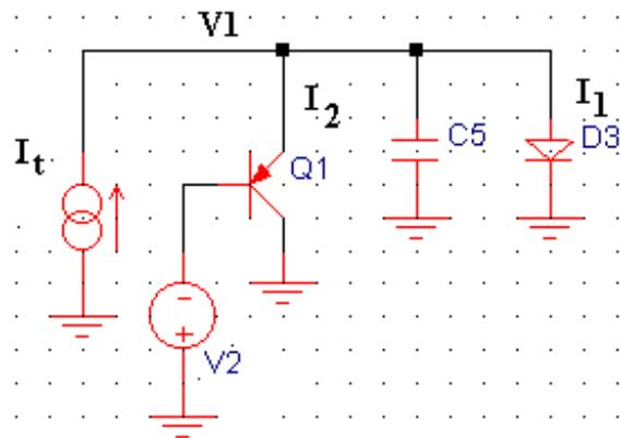
Figure 4. Transistor Shunt. V2 is < 200 mV.
