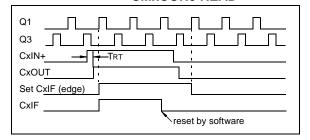
FIGURE 8-5: COMPARATOR INTERRUPT TIMING WITH CMxCON0 READ
