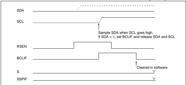
FIGURE 13-25: BUS COLLISION DURING REPEATED START CONDITION (CASE 2)
