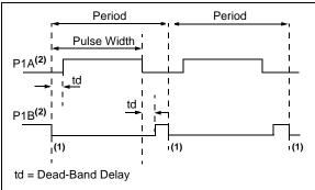
Note 1: At this time, the TMR2 register is equal to the PR2 register.
