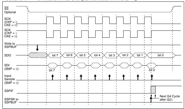
FIGURE 13-5: SPI MODE WAVEFORM (SLAVE MODE WITH CKE = 1)
