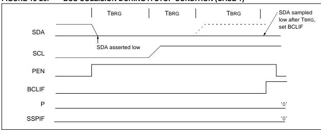
FIGURE 13-27: BUS COLLISION DURING A STOP CONDITION (CASE 2)
