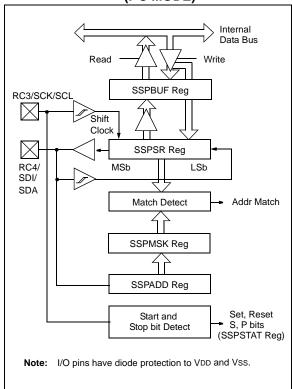
The MSSP module has these six registers for I<sup>2</sup>C operation:
