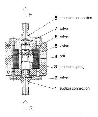
The piston (5) is moved by the electromagnetic field generated by the single wave diode rectified current flowing through the coil (4). Each current pulse moves the piston against the pressure spring (3). This movement, by reducing the volume in the suction chamber, opens the valve (6) set in the piston to let the liquid run to the pressure side.
