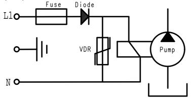
This electronic part must be mounted after the diode and the fuse, parallel to the pump (see electronic diagram). This mounting is necessary when the pump is stopped and started often by a commutator or a relay. The VDR will avoid the sticking of the commutator's contacts and protect the coil against a possible breakdown.
