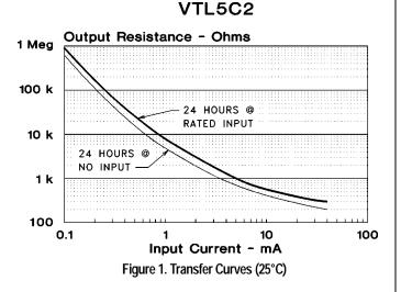
One of the characteristics of photocells is that their speed of response increases with increasing levels of illumination.<sup>1</sup> Thus the bandwidth of Vactrols is somewhat dependent upon the input drive level to the LED. In general, the higher the input drive the wider the bandwidth.
