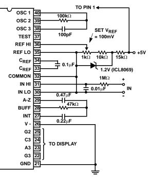
An external reference must be used in this application, since the voltage between V+ and V- is insufficient for correct operation of the internal reference.
