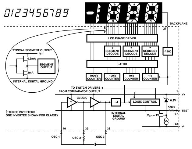
FIGURE 7. ICL7106 DIGITAL SECTION
