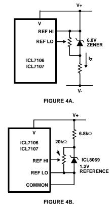
FIGURE 4. USING AN EXTERNAL REFERENCE
