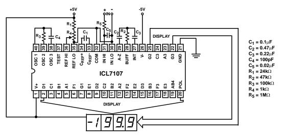
FIGURE 2. ICL7107 TEST CIRCUIT AND TYPICAL APPLICATION WITH LED DISPLAY COMPONENTS SELECTED FOR 200mV FULL SCALE
