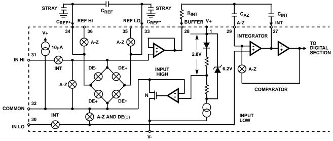
FIGURE 3. ANALOG SECTION OF ICL7106 AND ICL7107
