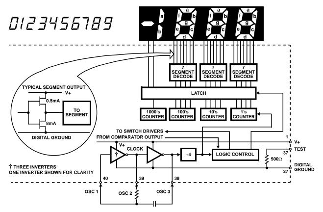
FIGURE 8. ICL7107 DIGITAL SECTION
