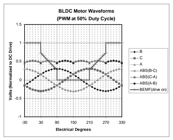
As expected the BEMF waveforms are all reduced proportionally but notice that the BEMF on the open terminal still equals half the applied voltage midway through the 60 degree drive phase. This occurs only when the drive voltage is on. Figure 10 shows a detail of the open terminal BEMF when the drive voltage is on and when the drive voltage is off. At various duty cycles, notice that the drive on curve always equals half the applied voltage at 60 degrees.
