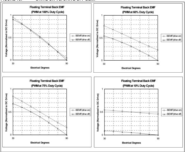
How well do the predictions match an actual motor? Figure 11 is shows the waveforms present on terminal A of a Pittman N2311A011 brushless motor at various PWM duty cycle configurations. The large transients, especially prevalent in the 100% duty cycle waveform, are due to flyback currents caused by the motor winding inductance.
