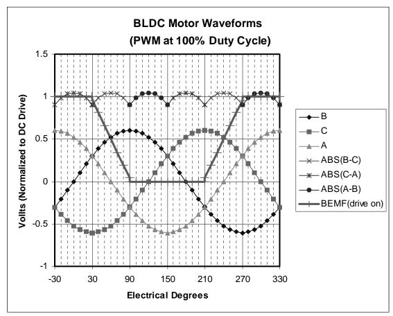
Notice that the BEMF(drive on) waveform is fairly linear and passes through a voltage that is exactly half of the applied voltage at precisely 60 degrees which coincides with the zero crossing of the coil A BEMF waveform. This implies that we can determine the rotor electrical position by detecting when the open terminal voltage equals half the applied voltage.
