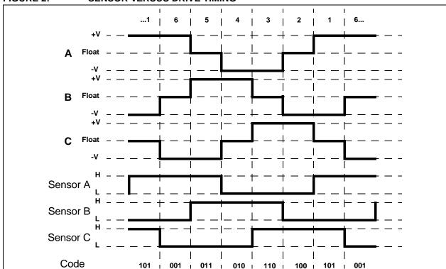
FIGURE 2: SENSOR VERSUS DRIVE TIMING
