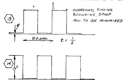
Vce must be no more than .2 volts with Vce being equal to 12V. Waveform must be symetrical respective to one another with a minimum of ringing and rounding of corners. The adverse conditions will increase as the load is increased.
