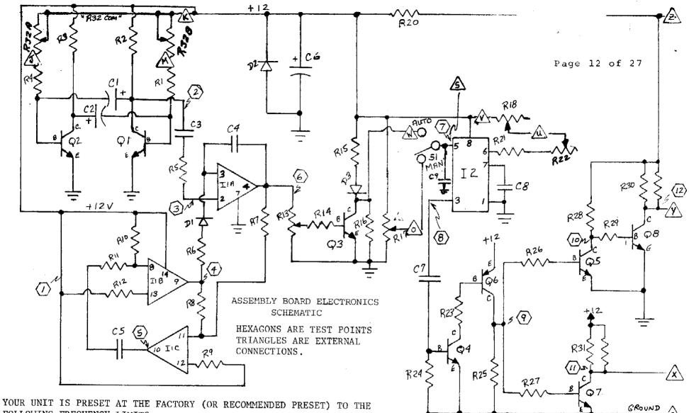
FOLLOWING FREQUENCY LIMITS: Range is 5Khz to 20Khz adjustable via R18 "MAIN FREQ CONTROL".
