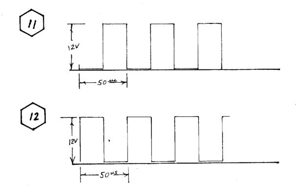
DRIVER OUTPUT TO BASE - THESE WAVE FORMS ARE 180 degrees OUT OF PHASE RESPECTIVE TO ONE ANOTHER (TEST POINTS AND (11 and 12) MUST SUPPLY SUFFI-CIENT CURRENT TO CAUSE COMPLETE SATURATION OF THE FINAL AMPLIFIER TRAN-SISTORS.
