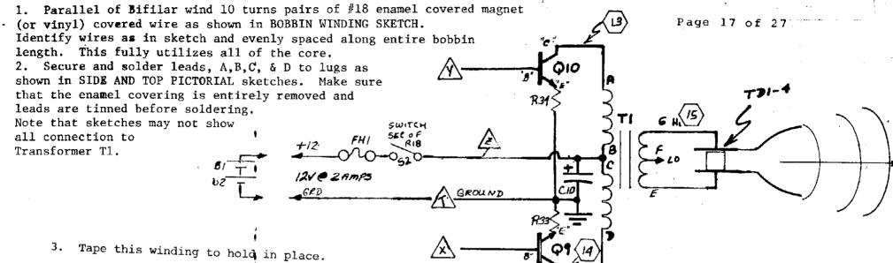
You may wish to bring out several taps on winding E & F to obtain optimum voltage levels for desired amount of transducers used. Rms voltage under load should be about 15 volts. Higher voltage and more output can be obtained for intermittent operation at the expense of possibly blowing transducers.
