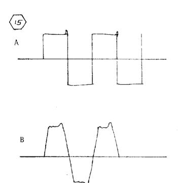
WAVESHAPE AT E & F WITHOUT TRANSDUCERS CONNECTED
