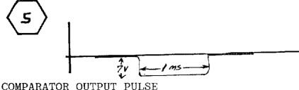
THIS MEASUREMENT IS UNNECESSARY IF WAVE FORM PICTURES 4 & 6 ARE OK INDI-CATING THE SCG STAGE IS PERFORMING CORRECTLY. IF NECESSARY, EXTERNAL TRIGGERING WILL BE REQUIRED - Use PIN 9 of 11B.
