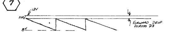
VCO OUTPUT WAVESHAPE - THE ABOVE WAVESHAPE VARIES FROM t=100 usec to 50 usec OR A CORRESPONDING FREQUENCY OF FROM 10KHZ TO 20KHZ, depending on Step 20 adjustments. NOTE SYMETRY OF THIS WAVESHAPE.
