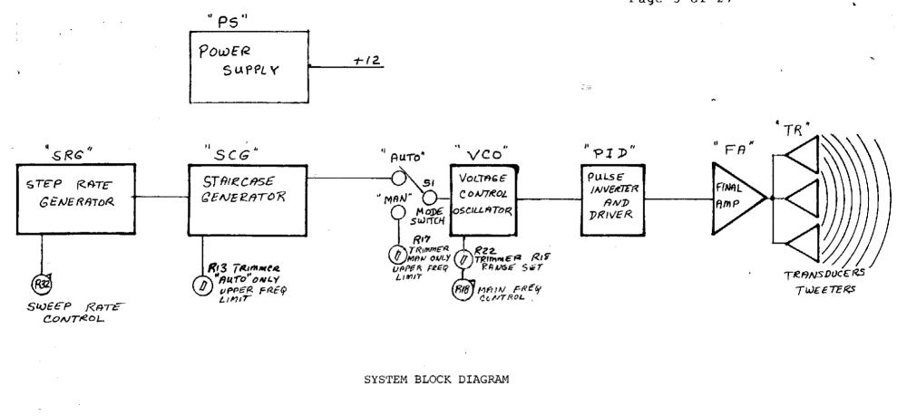
The power supply for this device can be any medium duty source of batteries developing 12Vdc. Plans show the use of  $8 - 1\frac{1}{2}$  "D" cells of the nickel cadmium variety connected in series for 12 volts. The Nicads are easily changed and reusable. Batteries may be replaced by a battery eliminator or conventional power supply capable of 2 amps at a low ripple rate.
