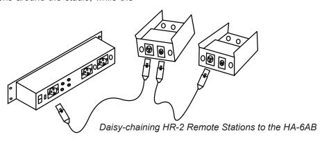
One or two sets of studio speakers may be connected to the HA-6AB. If two sets are needed, the "B" pair must be connected to the XLR output using a custom made cable. HR-2 Remote Stations cannot be used in this case.
