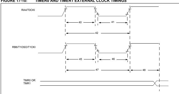
FIGURE 17-10: TIMERO AND TIMER1 EXTERNAL CLOCK TIMINGS
