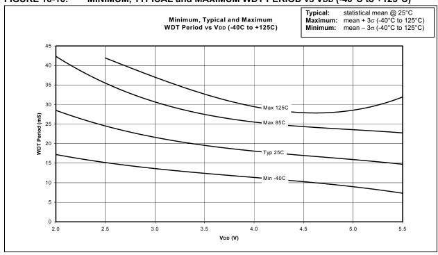
FIGURE 18-17: TYPICAL WDT PERIOD vs VDD (-40°C to +125°C)
