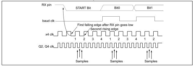
FIGURE 12-3: RX PIN SAMPLING SCHEME, BRGH = 1
