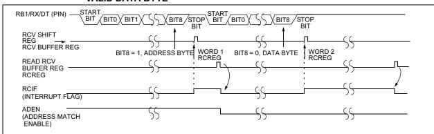
Note 1: This timing diagram shows an address byte followed by an data byte. The data byte is read into the RCREG (Receive Buffer) because ADEN was updated after an address match, and was cleared to a '0', so the contents of the Receive Shift Register (RSR) are read into the Receive Buffer regardless of the value of Bit 8.
