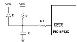
Note 1: External Power-on Reset circuit is required only if VDD power-up slope is too slow. The diode D helps discharge the capacitor quickly when VDD powers down.
