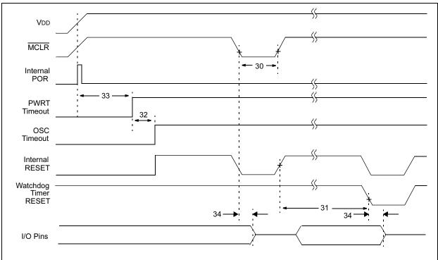
FIGURE 17-9: BROWN-OUT DETECT TIMING
