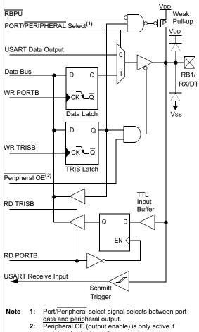
Peripheral OE (output enable) is only active if peripheral select is active.
