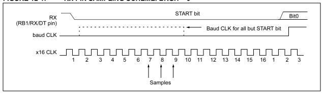
FIGURE 12-2: RX PIN SAMPLING SCHEME, BRGH = 1
