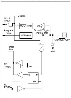
**BLOCK DIAGRAM OF** FIGURE 5-6: **RA6/OSC2/CLKOUT PIN**
