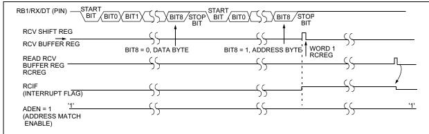
**Note** 1: This timing diagram shows a data byte followed by an address byte. The data byte is not read into the RCREG (Receive Buffer) because ADEN = 1 and Bit 8 = 0.
