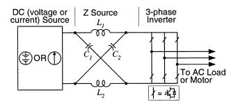
Fig. 4. Z-source converter structure using the antiparallel combination of switching device and diode.
