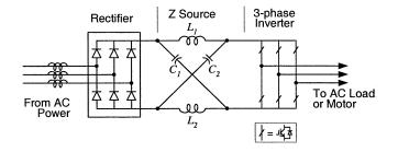
Fig. 17. Z-source rectifier/inverter system for adjustable-speed drives.
