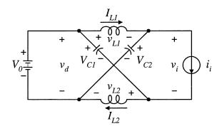
Fig. 10. Equivalent circuit of the Z-source inverter viewed from the dc link when the inverter bridge is in one of the eight nonshoot-through switching states.
