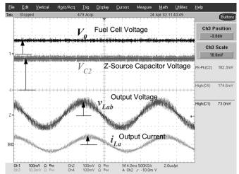
Fig. 15. Experimental waveforms when the fuel-cell voltage is low, inverter modulation index M = 0.642, and shoot-through period ratio  $T_0/T = 0.358$  ( $V_0$  and  $V_{C2}$  : 200V/div,  $V_{Lab}$  : 2\*;200V/div,  $i_{La}$ : 50 A/div, and time: 4 ms/div).
