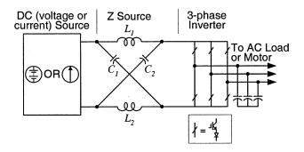
Fig. 5. Z-source converter structure using the series combination of switching device and diode.
