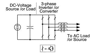
Fig. 1. Traditional V-source converter.
