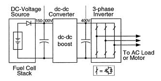
Fig. 6. Traditional two-stage power conversion for fuel-cell applications.
