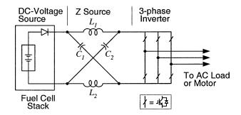
Fig. 7. Z-source inverter for fuel-cell applications.
