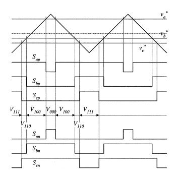
Fig. 11. Traditional carrier-based PWM control without shoot-through zero states, where the traditional zero states (vectors)  $V_{111}$  and  $V_{000}$  are generated every switching cycle and determined by the references.
