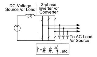
Fig. 2. Traditional I-source converter.
