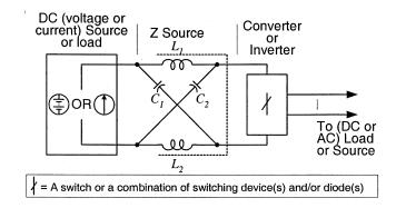
Fig. 3. General structure of the Z-source converter.
