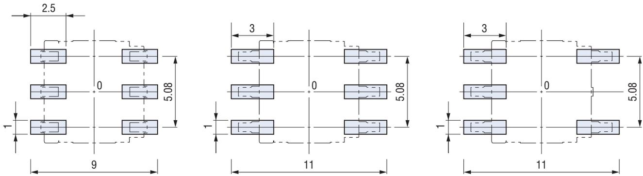
Note) The zero point is the center of mounting.
