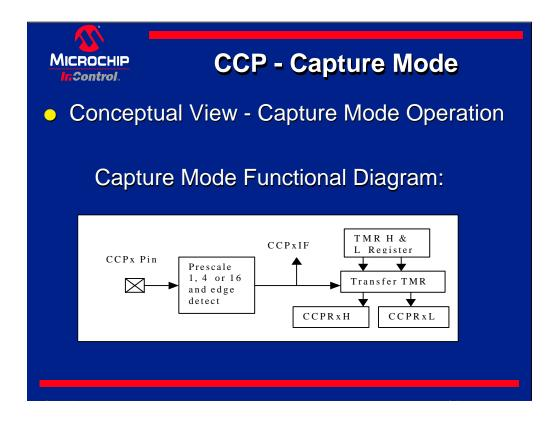
The capture mode functional diagram illustates how the incoming pulses are divided by the pre-scaler value before setting the CCPxIF flag, indicating a positive capture condition/event. The signal evaluated by the pre-scaler originates from the external CCPx pin and routed to the pre-scale circuitry. A pre-scaler is used to increase the number of edge counts required before sending the CCPxIF and transferring Timer high and low contents to CCPRxH and CCPRxL registers.
