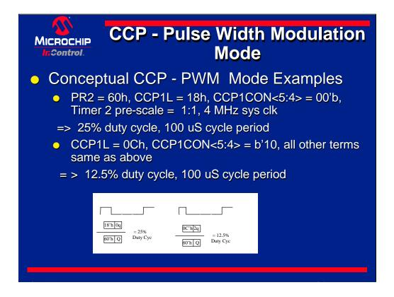
Conceptually, the proportional percentage of the duty cycle output is reflected by CCPxL to PR2.
