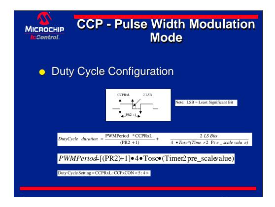
Duty cycle configuration for PWM operation.
