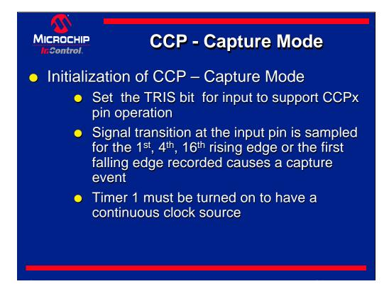
Before using the CCP module for operation, initialization of CCPx pin data direction, selection of CCP mode, and timer 1 or timer 2 setup and is required.
