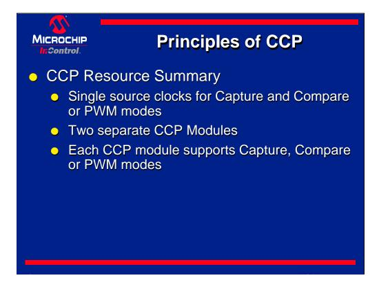
The mid-range Pic micro-controller can contain up to two CCP modules. Each module operates independently, and supports capture, compare or PWM mode. Operation is synchronized to internal clocks. A single clock source is shared between all available Capture and Compare or PWM CCP modules on chip.
