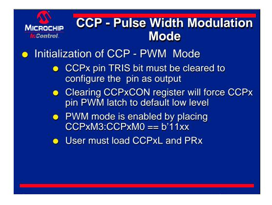
Initialization of CCP module for PWM operation required four steps:
