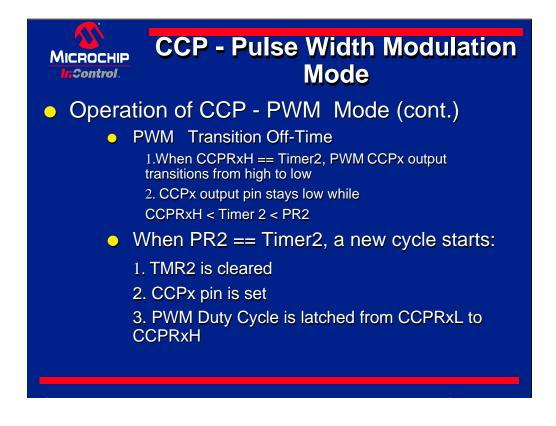
Reset cycle, started by CCPRxH equal to timer 2, causes PWM CCPx output to transition from high to low. CCPx pin will remain low while timer 2 is between CCPRxH and PR2 values.
