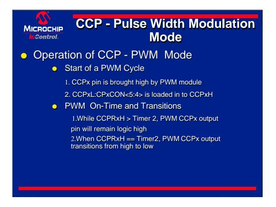
Operation of CCP module in PWM mode uses three main cycles: Start, Transition, and Restart
