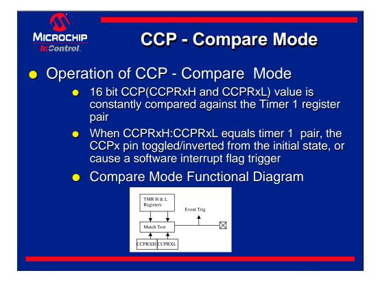
CCPx pin toggle event is driven by the match of a moving 16 bit counter, timer 1, against a known 16 bit value, cascaded CCPRxH and CCPxL value. When timer 1 equals CCPRx, a CCPx bit toggles, an interrupt or special event trigger occurs. The special event trigger output of CCP will cause a reset of timer 1 high and low bytes, and offer a means to start a conversion cycle in many mid-range parts containing an ADC module.
