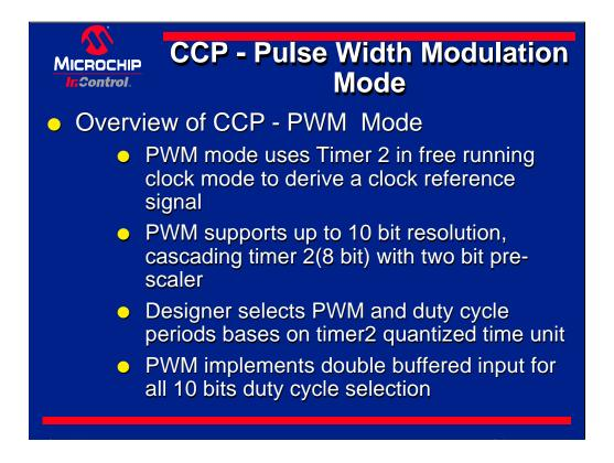
The CCP module supports a third mode, pulse width modulation(PWM). PWM module uses timer two in free running clock mode to derive a reference clock.
