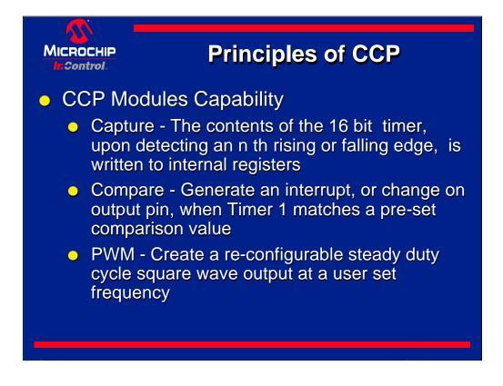
A capture, compare, and PWM, module, or CCP for short, is designed into the PicMicro to assist with measurement or control of time based pulse signals.
