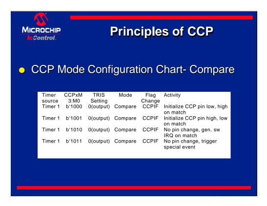
CCPxCON bits<3:2> equal to 10'b specifies compare mode, while bits<1:0> will determine the activity. The activity options consist of a low to high or high to low CCPx pin state change on match, software IRQ or special trigger on match. In Compare mode, for all activities, CCPIF flag will be set and timer 1 is used in free running mode.
