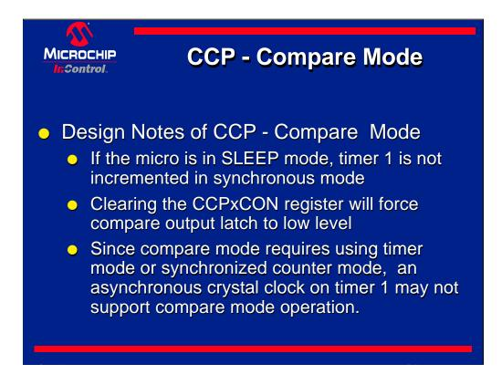
Since compare mode depends on timer one in synchronous mode, and timer one depends on system clock in synchronous mode, timer one will not increment, preventing compare mode from operating while PIC micro is in SLEEP mode.
