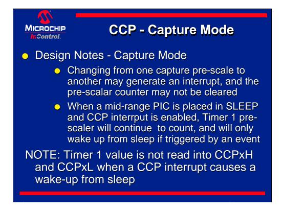
Changing from one capture pre-scale to another may generate an interrupt, and the pre-scaler counter may not be cleared. To prevent this from occurring, disable the CCP module before setting a new pre-scaler and returning back to capture mode.
