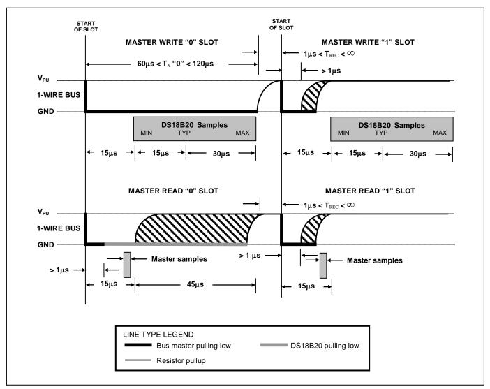
Figure 14. Read/Write Time Slot Timing Diagram
