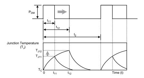
Figure 23: The Change in Junction Temperature due to Conduction Time
