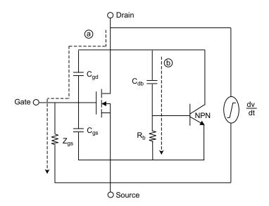
Figure 18: Equivalent Circuit of a N-channel MOSFET
