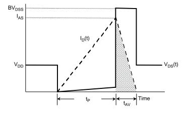
Figure 17: Unclamped Inductive Switching Waveforms.
