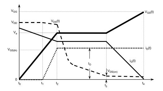
Figure 12: The Graph of  $V_{GS}(t)$ ,  $i_{G}(t)$ ,  $V_{DS}(t)$ ,  $i_{D}(t)$  when it is turned on
