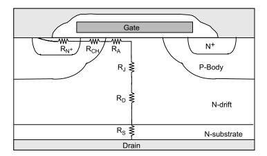
Figure 14: The Vertical Structure of a MOSFET Showing Internal Resistance
