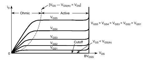
Figure 6: Output Characteristics
