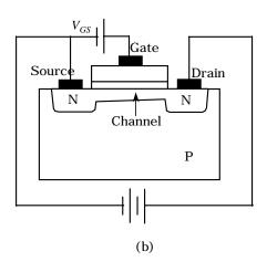
Figure 3: The Structure of an Enhancement Type MOSFET and its Operation
