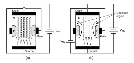
Figure 1: The Structure of a JFET and its Operation
