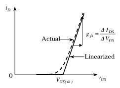
Figure 15: Transfer Curve & gfs
