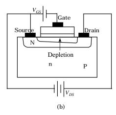
Figure 2: The Structure of a Depletion Type MOSFET and its Operation
