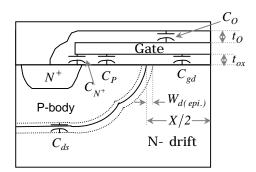
Figure 10: Vertical Structure Showing Parasitic Capacitance
