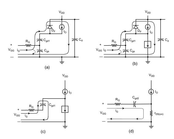
Figure 13: Equivalent Circuits of the MOSFET with Turn-on Divided into 4 Periods at the Diode-clamped Inductive Load Circuit.
