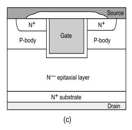
Figure 4: Vertical Channel Structure
