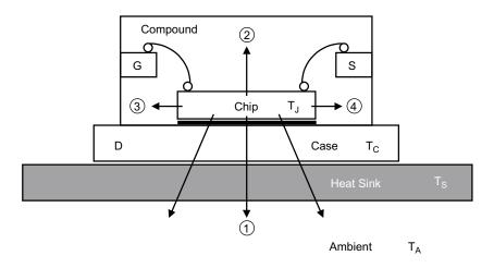
Figure 21: The Path of Thermal Discharge at the Chip Junction
