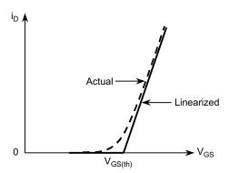
Figure 7: Transfer Curve
