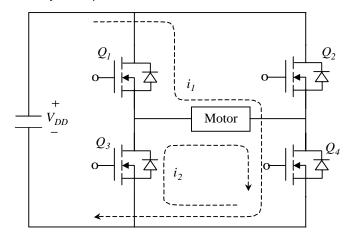
**Figure 19: Motor Control Circuit**
