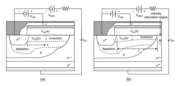
Figure 9: Inversion Layer Thickness Changes due to the Increase of the Drain-to-Source Voltage ( $V_{DD}$ ). Where,  $V_{DD1} < V_{GS} - V_{GS(th)}$ ,  $V_{DD2} > V_{GS} - V_{GS(th)}$ ,  $I_{D2}$  (saturation current)  $> I_{D1}$
