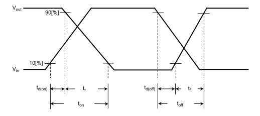
Figure 16: Resistive Switching Waveforms
