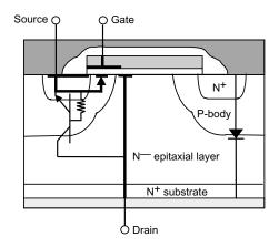
Figure 5: The MOSFET Vertical Structure Showing the Parasitic BJT and Diode
