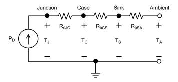
Figure 22: An Equivalent Circuit Based on Thermal Resistance
