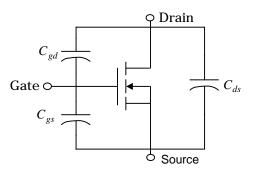
Figure 11: Equivalent Circuit Showing Parasitic Capacitance
