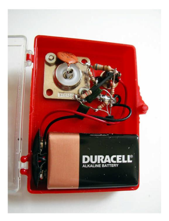
Simple point-to-point wiring is used. No printed circuit board is required. Short, direct leads produce the best noise spectrum. Unwanted capacitance to a ground plane or excessive lead lengths will produce an uneven noise spectrum and limit the upper frequency of useful noise. This generator produces good noise throughout the HF spectrum and into the lower VHF range.
