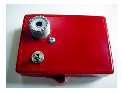
The simple generator is based on a circuit provided by Tom Hammond, N0SS. It is housed in a 3 in X 2 in X 3/4- in (75mm x 52 mm X 20 mm) plastic box.. The only operating control is the On/Off switch.
