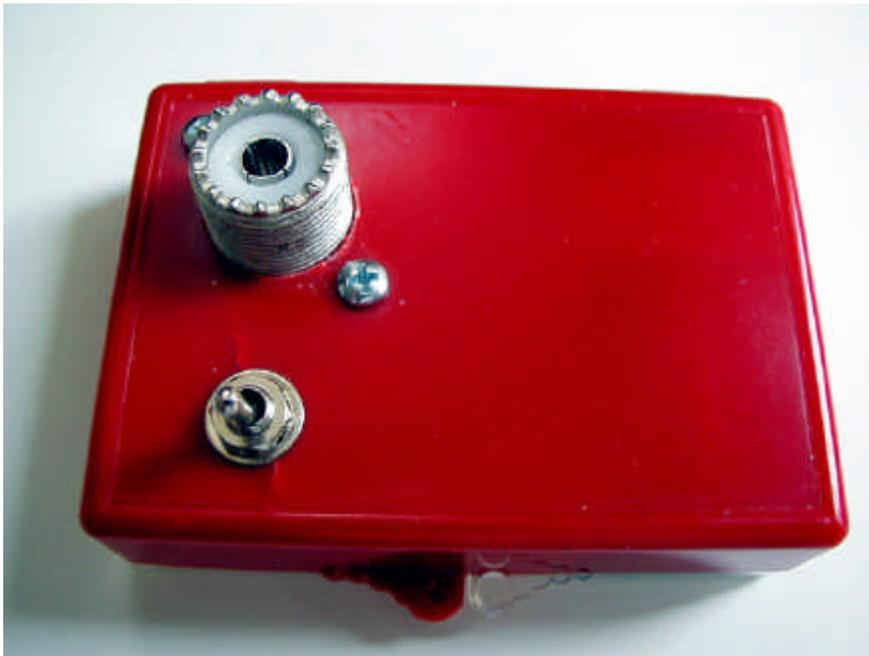
The simple generator is based on a circuit provided by Tom Hammond, N0SS. It is housed in a 3 in X 2 in X 3/4- in (75mm x 52 mm X 20 mm) plastic box.. The only operating control is the On/Off switch.
