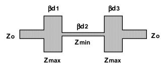
As a worked example, consider the design of a maximally flat three-section lowpass filter that has a cutoff frequency of  $f_c = 1$  GHz. The highest practical impedance is  $Z_{max} = 120$  ohms and the lowest practical impedance is  $Z_{min} = 12$  ohms. Assume we have
