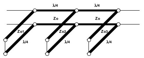
This filter can also be configured as a bandstop filter by using open rather than shorted stubs. While it's easy to see that this filter will pass the center frequency for which the lines are all  $\lambda/4$ , we would like to be able to design such a filter using lumped element prototypes.
