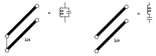
But it is important to note that a parallel tuned circuit is transformed through a  $\lambda/4$  line to the impedance of a series tuned circuit, and vice versa. This allows us to determine the equivalent circuit of the transmission line filter.
