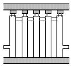
One major benefit of the combline filter is that, uniquely among the forms shown above, it can be designed so that the interplay of distributed and lumped elements can be used to eliminate the higher order passbands. As we will see in later lectures, this is a very significant advantage for large-signal circuits that have substantial harmonic energy.
