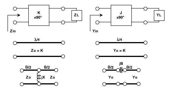
For the impedance inverter,  $Z_{in} = K^2/Z_L$
