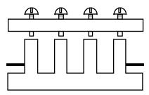
Consider a filter such as a comb-line filter which has been designed but must now be tuned. If all the tuning screws are shorted to their respective resonators, the output admittance at, say, the input port plane is very high. As that resonator is tuned, the reflection coefficient stays high because the rest of the filter is still shorted, but the phase of the reflection coefficient can range through a 180° range. If we stop at 90° phase
