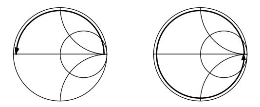
When we tune the last resonator, we see the load at the output of the filter. But we can still get the proper tuning by observing the additional 90° phase change.
