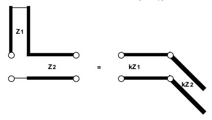
This diagram shows the equivalence for the most commonly used identity, which removes a series stub by transforming it to a shunt stub along with adjustment of characteristic impedances of the  $\lambda/8$  lines.
