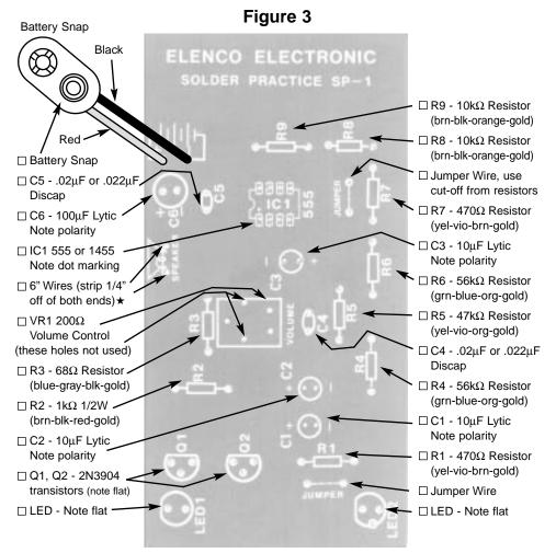
$\square$  After completing the above assembly, twist the two speaker wires together and solder to speaker lugs.
