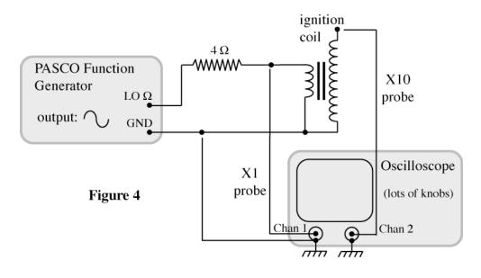
11. How could you determine the turns ratio for your particular coil? Briefly describe what you would do to measure the turns ratio. Proceed with your measurement after checking with your instructor. What is the turns ratio?
