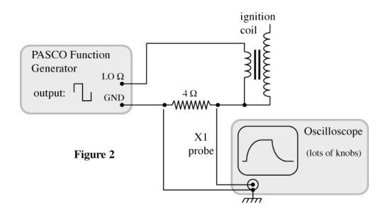
4. How long does it take for the current to build up to close to its maximum value? To 63% of the maximum? How long does it take to decay to 37% of the maximum? To zero?
