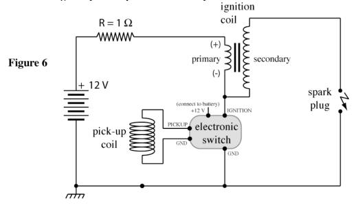
Connect the pick-up coil and electronic switch (the green circuit board) to the rest of the ignition circuit as shown in Figure 6. Often not all wires are shown in a circuit diagram to help make the functionality of the circuit more clear; in this case the wire that connects the battery to the electronic switch (the electronic switch needs battery power to operate) is not drawn in. All ground (GND) connections on the circuit board are in common (are connected together).
