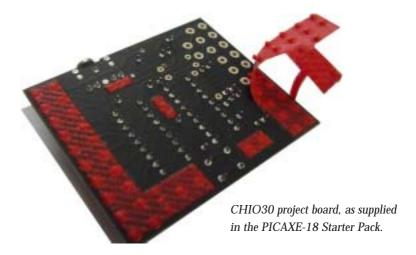
This peelable layer protects the user solderable pads during manufacture and storage, to keep the pads clean and grease free.
