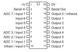
Note pin C.6 is **input only** on the 20M2 and 20X2 parts. This is due to the internal silicon design of the chip and cannot be altered.
