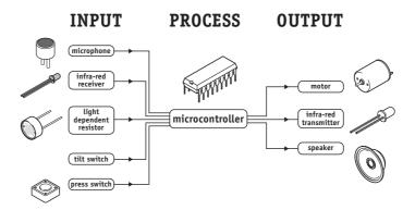
The microcontroller uses information from the input transducers to make decisions about how to control the output devices. These decisions are made by the control program, which is downloaded into the microcontroller. To change the 'behaviour' of the toy it is simply a process of changing and downloading a new program into the microcontroller
