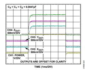
Figure 22. Typical Turn-On Time,  $V_S = 3 V$
