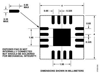
Figure 26. Recommended PCB Layout
