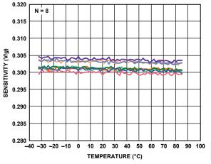
Figure 18. X-Axis Sensitivity vs. Temperature— Eight Parts Soldered to PCB, V<sub>S</sub> = 3 V
