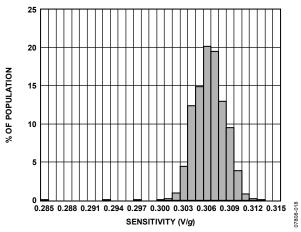
Figure 16. Y-Axis Sensitivity at 25°C,  $V_S = 3 V$
