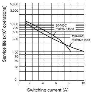
Note: The 120 VAC resistive load service life curve also applies for 250 VAC resistive load.
