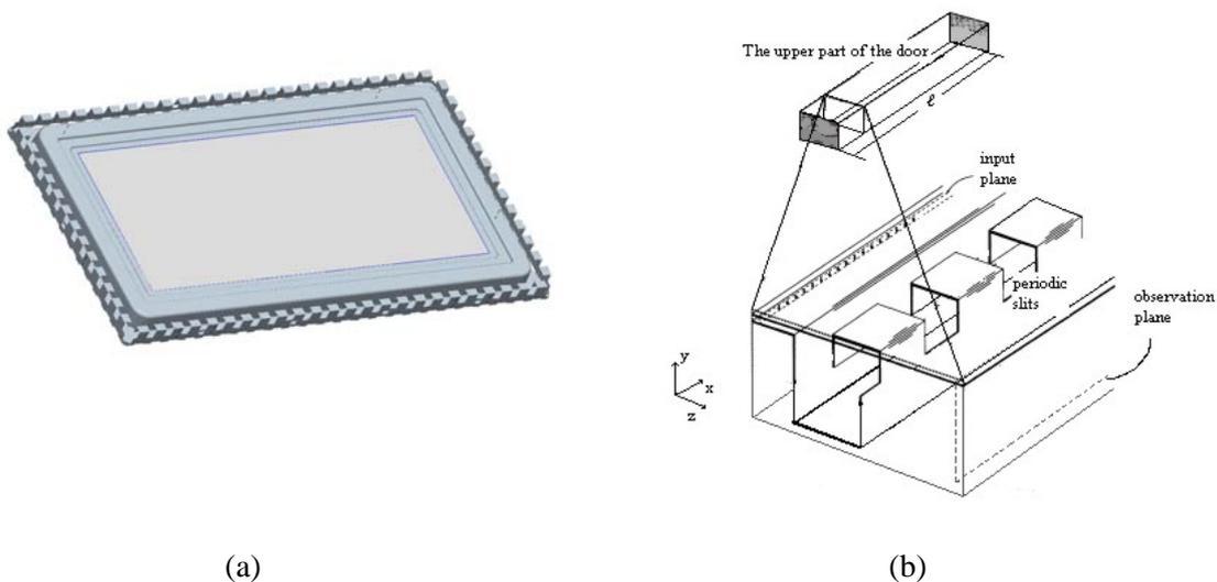
Fig. 1 - (a) Microwave oven door and (b) computational model of the door seal structure
