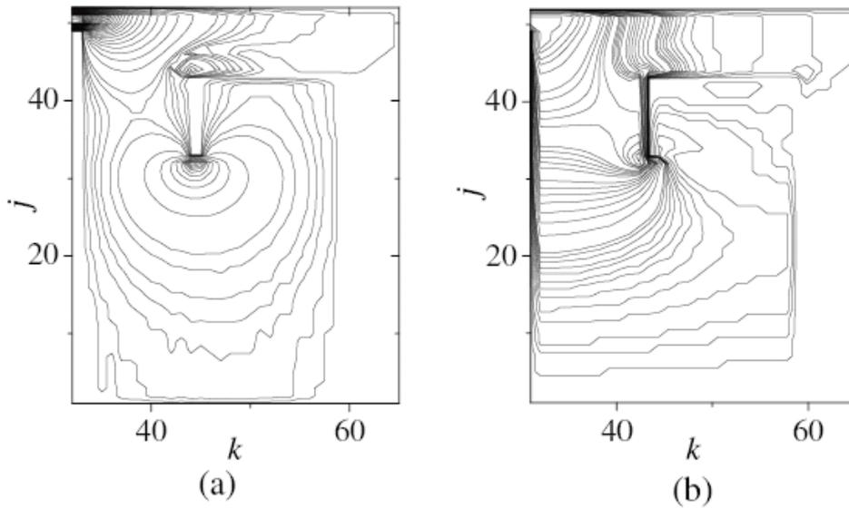
Fig. 3 – (a) Absolute value of the electric field and (a) radiation intensity inside the choke structure
