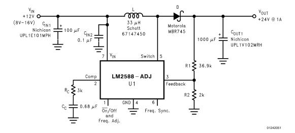
FIGURE 38. +12V to +24V Boost Regulator
