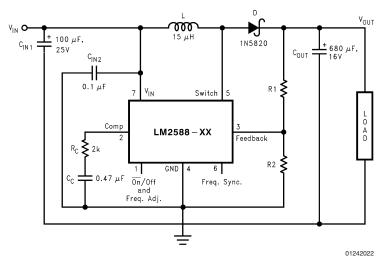
$C_{IN1}-100~\mu F$ , 25V Aluminum Electrolytic $C_{IN2}-0.1~\mu F$  CeramicL  $-15~\mu H$ , Renco #RL-5472-5D  $-18820C_{OUT}-680~\mu F$ , 16V Aluminum Electrolytic $C_{C}-0.47~\mu F$  CeramicR $_{C}-2k F$ or 12V Devices: R1 = Short  $(0\Omega)$  and R2 = OpenFor ADJ Devices: R1 = 48.75k,  $\pm 0.1\%$  and R2 = 5.62k,  $\pm 0.1\%$
