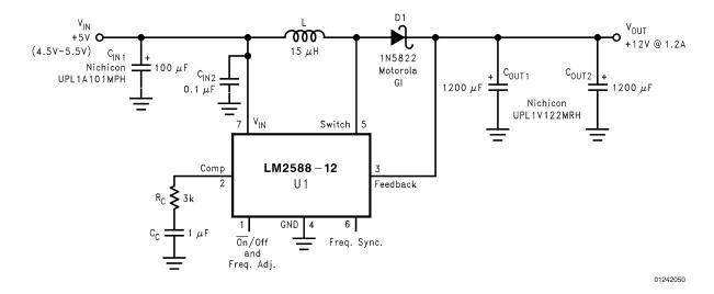
FIGURE 36. +5V to +12V Boost Regulator
