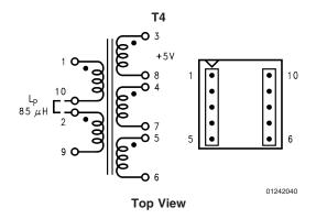
FIGURE 24. Pulse PE-68422 (Surface Mount)
