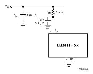
FIGURE 47. Input Line Filter
