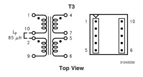
FIGURE 23. Pulse PE-68421 (Surface Mount)
