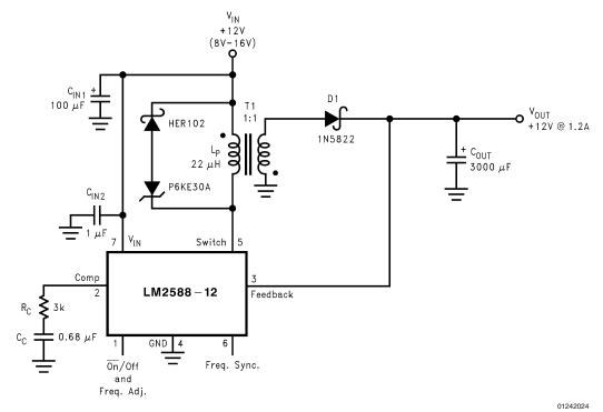
As shown in Figure 4, the LM2588 can be used as a flyback regulator by using a minimum number of external components. The switching waveforms of this regulator are shown in Figure 5. Typical Performance Characteristics observed during the operation of this circuit are shown in Figure 6.
