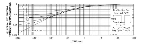
Figure 11. Transient Thermal Response Curve.
