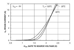
Figure 5. Transfer Characteristics.
