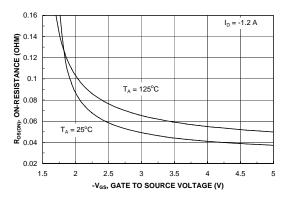
Figure 4. On-Resistance Variation with Gate-to-Source Voltage.
