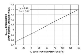
Figure 3. On-Resistance Variation with Temperature.
