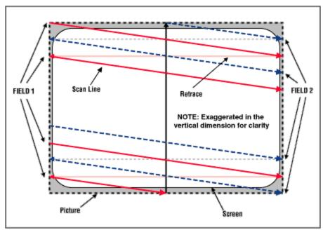
Figure 2. Interlaced scanning system.
