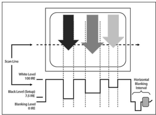
Figure 1. Horizontal scan versus display brightness.
