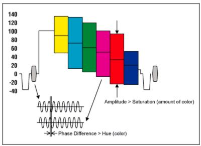
Figure 6. Composite video waveform: color bars.
