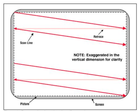
Figure 3. Progressive (non-interlaced) scanning system.
