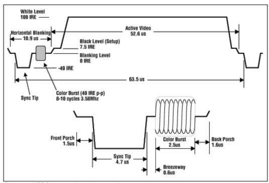
Figure 5. NTSC composite video waveform.
