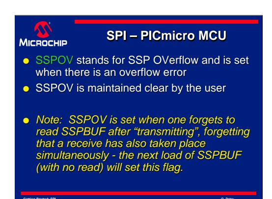
As mentioned previously, SSPOV means "Synchronous Serial Port OVerflow" and is set by the microcontroller whenever there is an overflow error.
