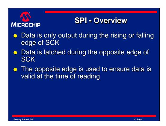
In SPI, data typically changes during the rising or falling edge of SCK. This is how the data is synchronized with the clock signal.
