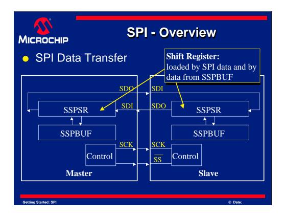
SSPSR is the shift register for the SPI module. It shifts data in and out of the device. The data travels in a loop to the next shift register. The data is shifted out the SDO pin of one device and into the SDI pin of the other.
