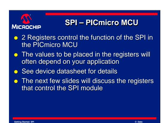
When using SPI in the PICmicro device, a few registers need to be set up correctly. Two registers run the SPI engine itself, which we will discuss next.
