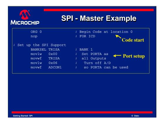
The code starts at "ORG 0". The ORG is a directive to MPLAB and stands for "ORiGin" and tells the assembler where in program memory to locate the next instruction. Any time an "ORG" is encountered, the next program memory instruction will begin at the new location. In this example, the program will begin at 0, while the next instruction will be at program memory location 1, then 2 and so on.
