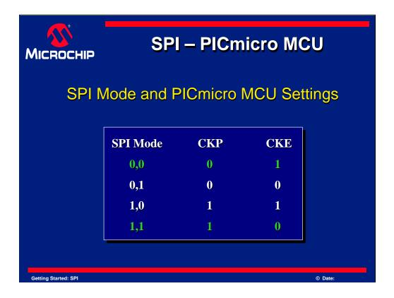
Here is a diagram of what to set CKP and CKE to for any desired SPI mode. The values in green represent the most commonly used configurations of SPI.
