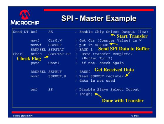
The next line of code sets the Slave Select (SS) line low. This will enable the SS line on the slave, which will tell it an SPI transfer is about to occur.
