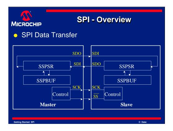
SPI creates a data loop between two devices. Data leaving the master exits on the SDO (serial data output) line. Data entering the master enters on the serial data input, SDI line.
