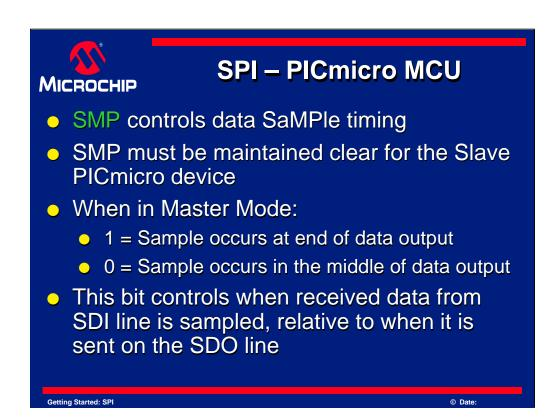
SMP controls the data SaMPle timing.
