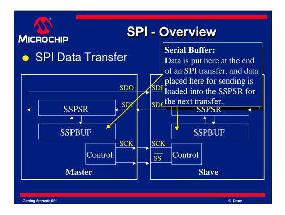
Once a byte of data has been exchanged between the two devices, it is copied to the SSPBUF register. The SSPBUF is then read by the user software.
