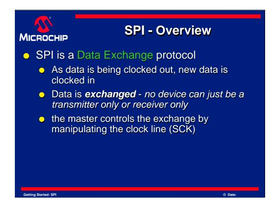
SPI is a Data Exchange protocol. As data is being clocked out, new data is also being clocked in.
