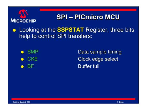
The next register that controls SPI is the SSPSTAT register. SSPSTAT stands for "Synchronous Serial Port STATus" and provides a few bits for controlling the SPI communication.
