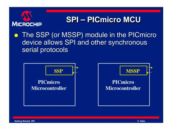
In the PICmicro device, a module is used for the SPI protocol. This module is named the SSP or MSSP module and allows SPI or I<sup>2</sup>C to be implemented.
