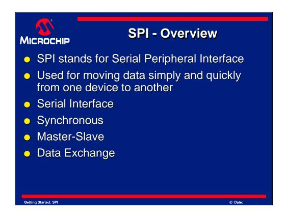
SPI stands for Serial Peripheral Interface.
