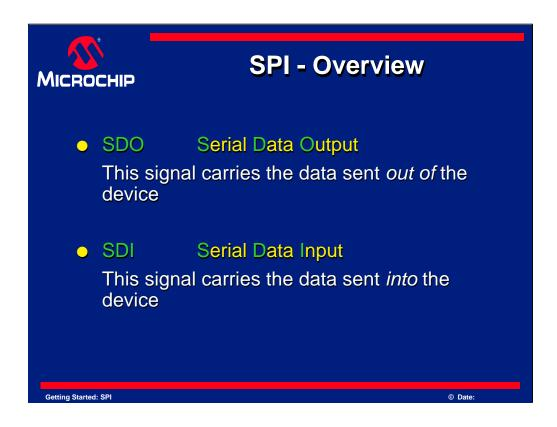
SDO - This is the Serial Data Output signal. SDO carries data out of a device.
