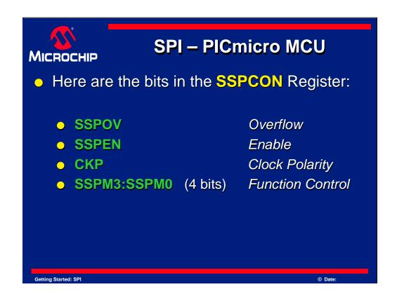
The SSPCON register one other register that controls the SPI engine.
