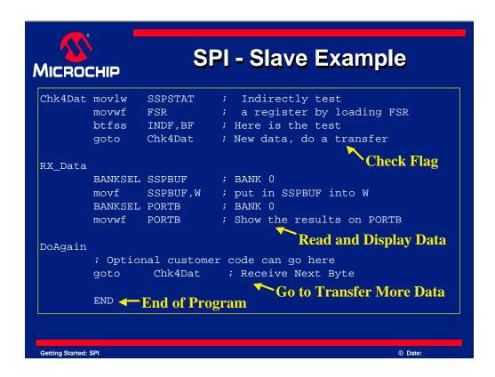
This is the loop that looks for SPI data. The BF flag is tested and when it is set, the data is obtained from the SSPBUF register.
