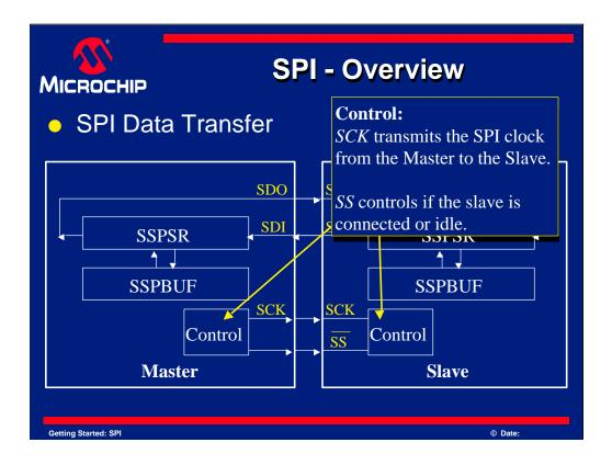
The control block determines when an SPI transfer can take place. When referring to the master device this section transmits a clock and slave select signal. The slave device waits for these signals and uses them when processing the SPI data.
