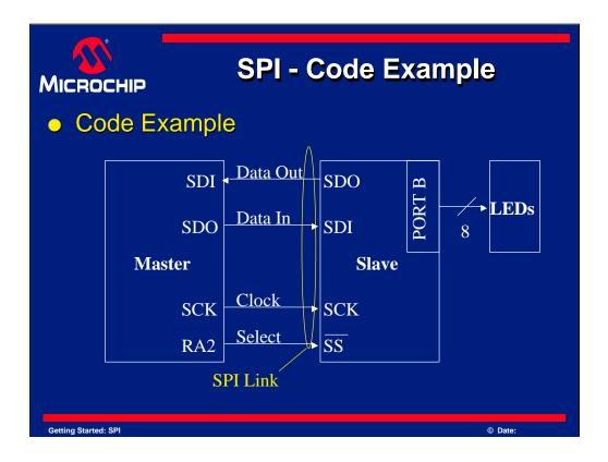
Here is a simplified schematic of what is done in this example. An SPI link is set up between the Master and Slave PICmicro devices. Then PORTB on the Slave PICmicro device is used to send data to eight LEDs.
