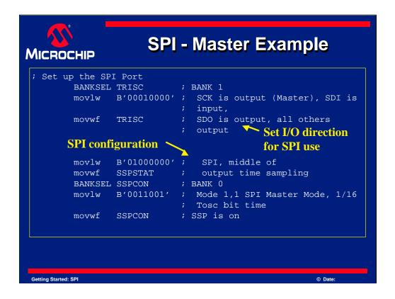
The next piece of code will set up PORTC. Notice that it has been configured so that SCK is an output, SDO is also an output, and SDI is an input. All other pins are configured as outputs. For this example, the other pins are not used.
