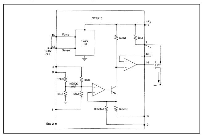
FIGURE 54. Precision single-supply voltage-to-current source transmitter—the XTR110.
