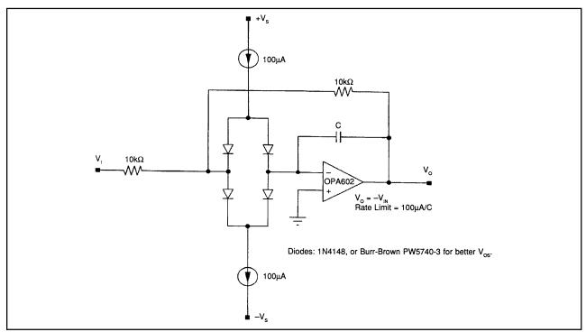
FIGURE 48. Rate limiting circuit.
