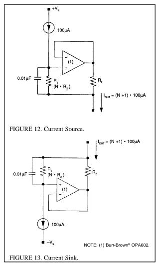
FIGURES 12 and 13. For a programmable current source with any output current greater than  $100\mu A$  and compliance to  $+V_s$  or -  $V_s,$  use a  $100\mu A$  current source as a reference along with an external op amp and two programming resistors.
