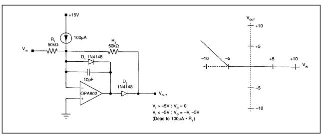
FIGURE 39. Precision positive dead-band circuit.
