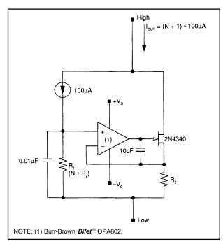
FIGURE 16. Use a 100µA Current Source as a reference, an external op amp, two programming resistors, and a series pass element for a programmable floating curent source.
