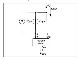
FIGURE 11. The two 100μA Current Sources and Mirror in the REF200 can be connected to form a 400μA floating current source.
