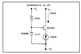
FIGURE 24. Cascoded Current Sink with compliance to  $-V_s+5V$  (using zener diode for bias).
