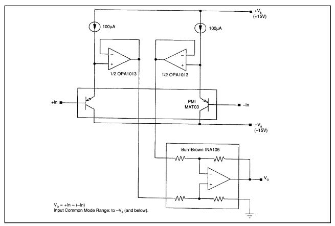
FIGURE 49. Single-supply instrumentation amplifier.
