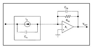
FIGURE 58. Virtual ground current-to-voltage converter.
