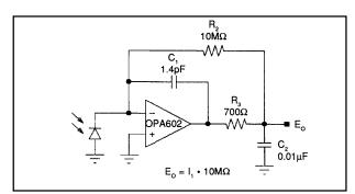
FIGURE 61. Improved transimpedance photodiode amplifier.
