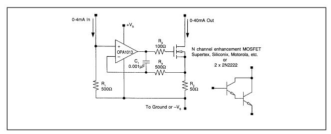
FIGURE 18. Sinking Current Mirror using series pass device.
