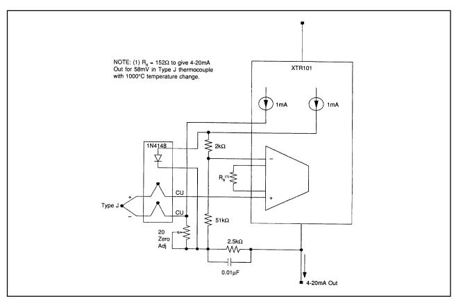
FIGURE 53. Temperature-controlled current source using XTR101.
