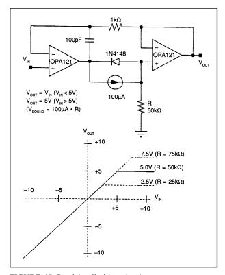
FIGURE 45. Precision limiting circuit.
