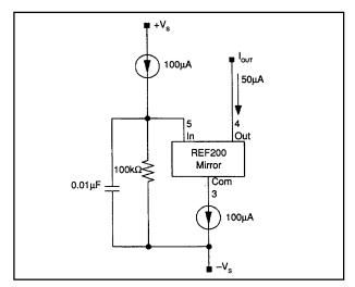
FIGURE 6. Compliance of the  $50\mu A$  Current Sink (Figure 5) can be extended to  $-V_s+5V$  by referencing its bias point to the negative power supply rail using the other  $100\mu A$  current and a resistor.
