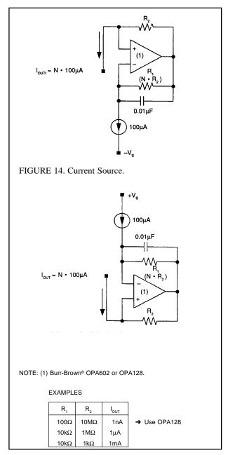
FIGURES 14 and 15. If you don't need compliance to the power supply rail, this circuit using a 100μA current source as a reference along with an external op amp and two programming resistors can provide virtually any output current.
