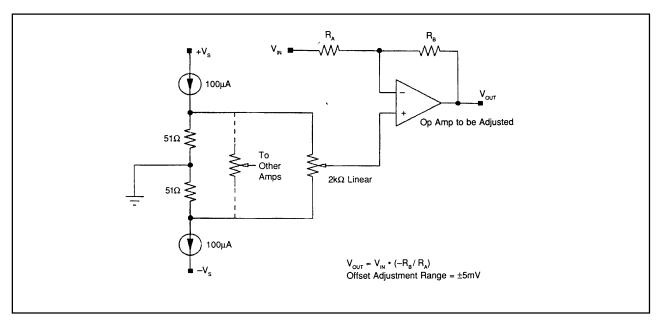
FIGURE 35. Op Amp Offset Adjustment Circuit uses the two 100μA current sources from a REF200 to provide accurate ±5mV references.
