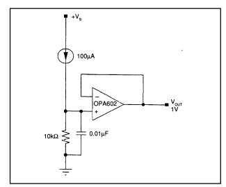
FIGURE 34. Buffered Voltage Reference.
