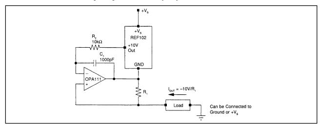
FIGURE 15B. Current Sink using Voltage Reference and Op Amp.
