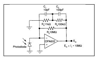
FIGURE 60A. Standard Transimpedance Amplifier with capacitor divider and added feedback pole.
