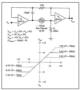
FIGURE 44. Precision double limiting circuit.
