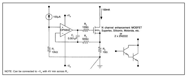
FIGURE 17. Programmable Current Sink using series pass device.
