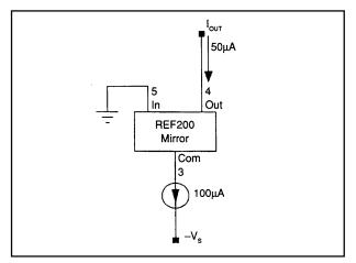
FIGURE 4. A 50µA Current Sink with compliance to ground can be made using one of the 100µA current sources and the mirror from the REF200.
