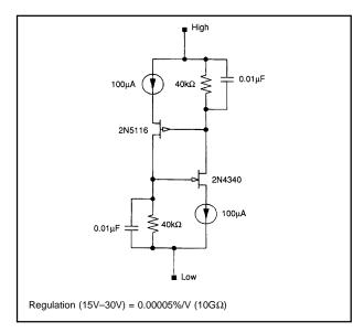
FIGURE 28. Cascoded 200µA Floating Current Source.
