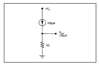
FIGURE 33. 100µV Reference for VFC off-zeroing.
