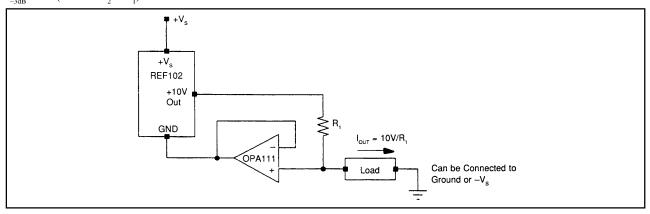
FIGURE 15A. Current Source using Voltage Reference and Op Amp.
