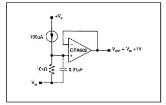
FIGURE 34A. Floating Voltage Reference.
