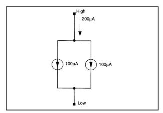
FIGURE 8. For a 200μA Floating Current Source simply parallel the two 100μA current sources from the REF200.
