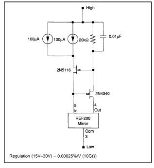
FIGURE 30. Cascoded 400µA Floating Current Source.
