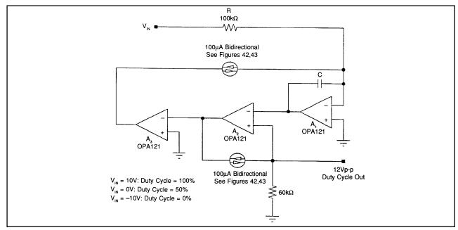
FIGURE 47. Precision duty-cycle modulation circuit.
