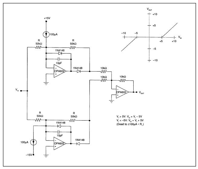
FIGURE 41. Precision double dead-band circuit.
