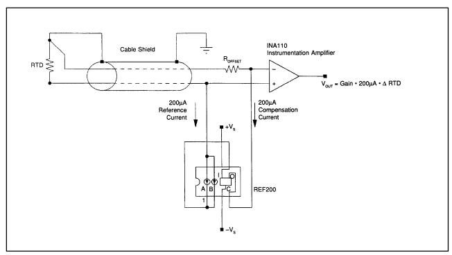
FIGURE 38. RTD excitation with three-wire lead resistance compensation.
