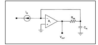
FIGURE 59. Virtual ground current-to-voltage converter redrawn to Illustrate phase delay due to input capacitance and feedback resistor.
