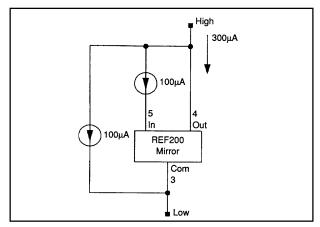
FIGURE 10. The two 100 $\mu$ A Current Sources and Mirror in the REF200 can be connected to form a 300 $\mu$ A floating current source.
