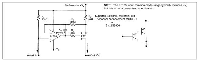
FIGURE 20. Sourcing Current Mirror using series pass device.
