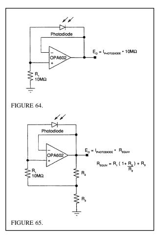
FIGURES 64 and 65. Photodiode amplifier using floating virtual ground current-to-voltage converter.
