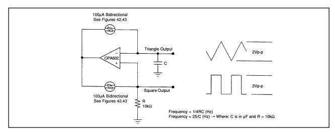
FIGURE 46. Precision triangle waveform generator.
