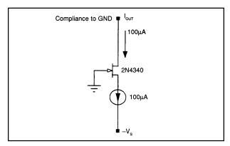
FIGURE 22. Cascoded Current Sink with compliance to ground.
