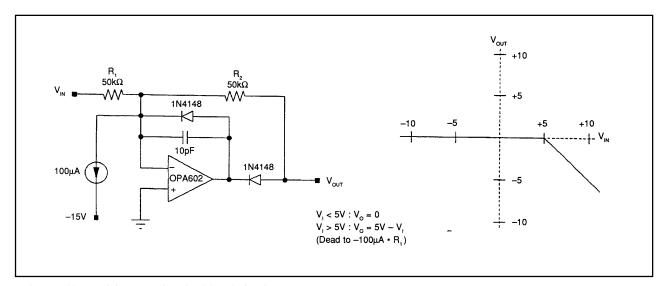
FIGURE 40. Precision negative dead-band circuit.
