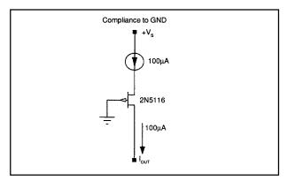
FIGURE 25. Cascoded Current Source with compliance to ground.
