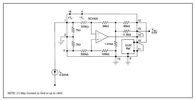
FIGURE 57. 4-20mA current loop receiver using the RCV420.
