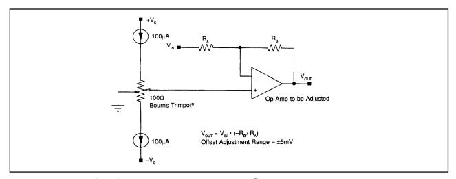
FIGURE 36. Op amp offset adjustment circuit using Bourns Trimpot®.
