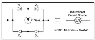
FIGURE 42. Bidirectional current source.
