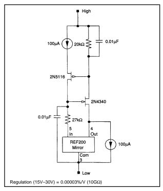
FIGURE 29. Cascoded 300µA Floating Current Source.
