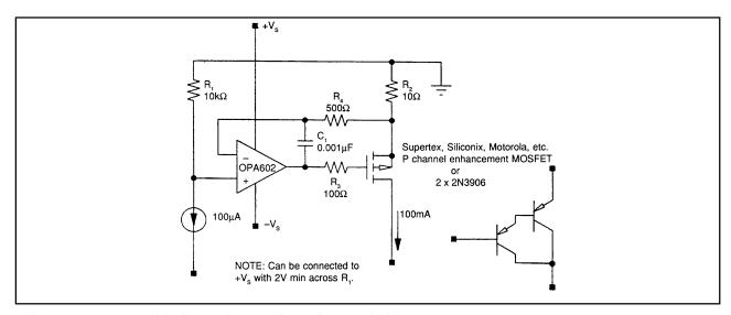
FIGURE 19. Programmable Current Source using series pass device.
