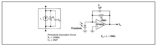
FIGURE 60. Standard transimpedance photodiode amplifier.
