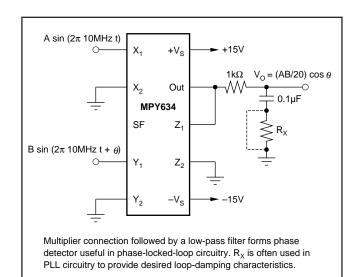
FIGURE 6. Phase Detector.
