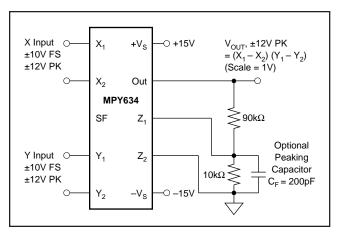
FIGURE 1. Connections for Scale-Factor of Unity.
