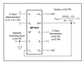
FIGURE 4. Basic Divider Connection.
