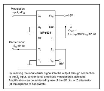
FIGURE 9. Linear AM Modulator.
