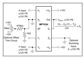
FIGURE 2. Basic Multiplier Connection.
