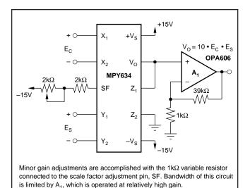
FIGURE 7. Voltage-Controlled Amplifier.
