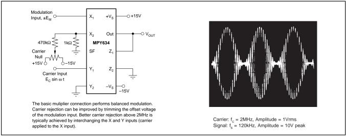
FIGURE 11. Balanced Modulator.
