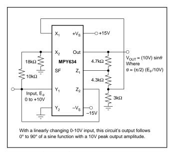
FIGURE 8. Sine-Function Generator.
