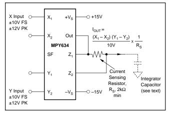
FIGURE 3. Conversion of Output to Current.
