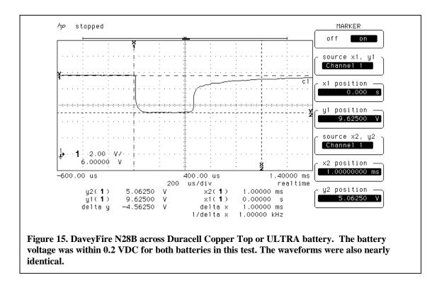
Last, we test the loading effects of a Robby's Rockets AG-1 Flashbulb-based ejection charge on a Duracell 9 VDC battery. The results are shown in figure 15. Notice how the voltage dips instantaneously from 9.65 VDC to 4.312 VDC. Depend on the avionics, this low voltage could cause anomalous behavior in some systems.
